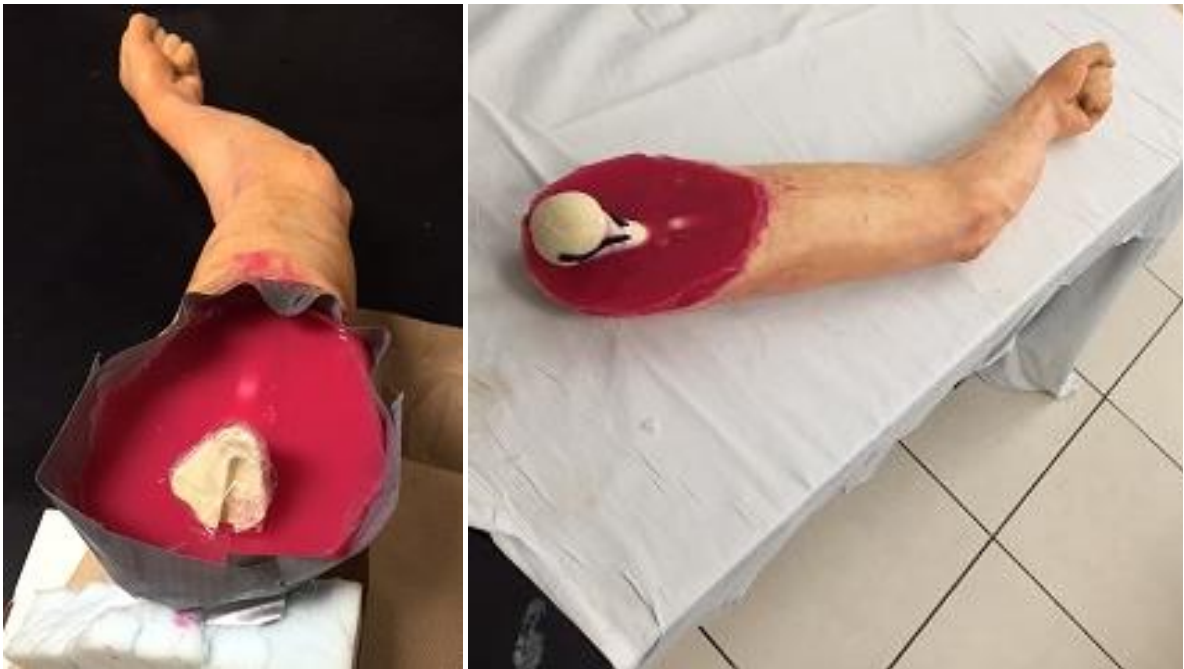
Figure 3.12: Arm with humerus inserted and sealed using silicone.
