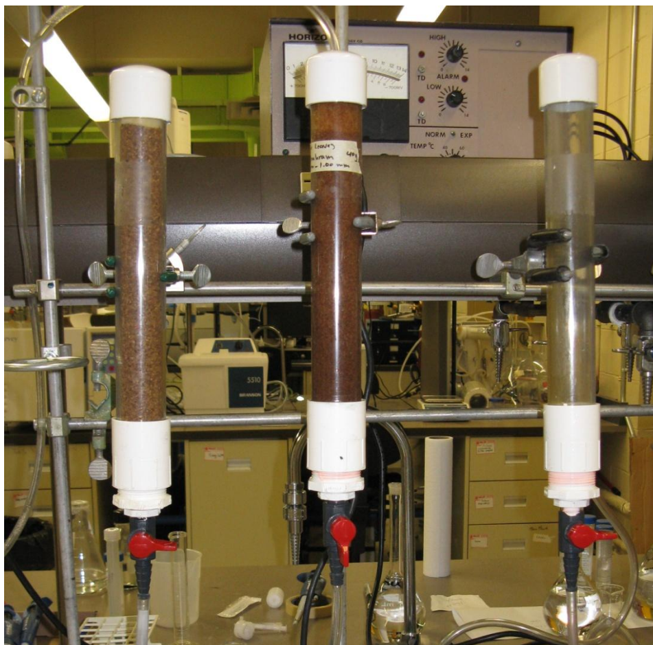
Figure 1.4. Experimental set-up for removal of heavy metals by maple leaves biomass in packed-bed columns.
