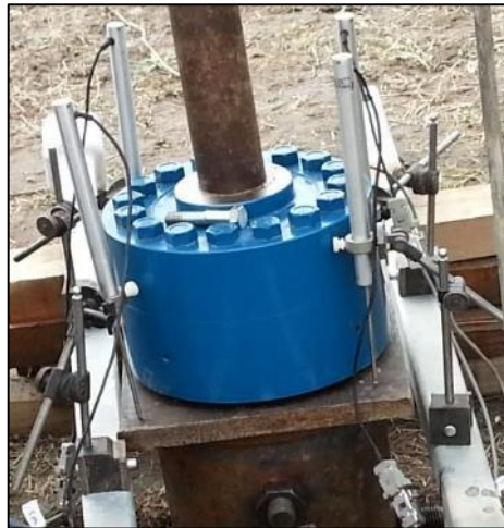
Figure 6 - 8: The used setup for (a) compressive testing; and (b) uplift testing
