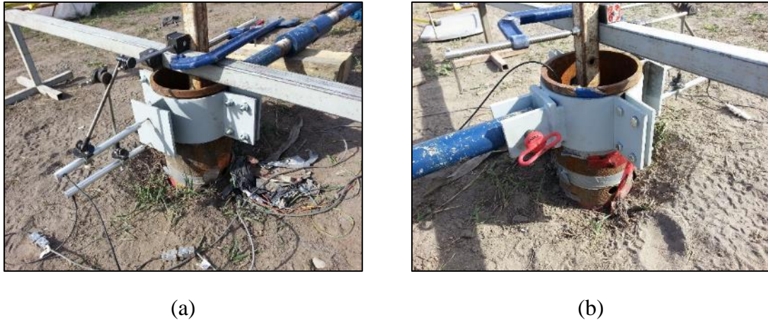
Figure 5 - 8: Lateral load setup components (a) steel clamp/LVDT plate, (b) clamp-rod connection
