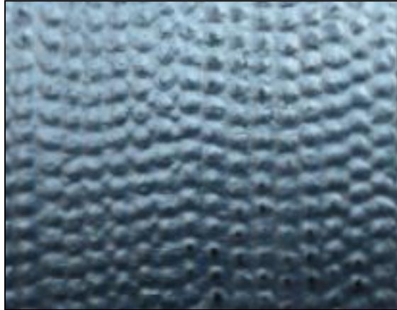
Figure 8 - 2: Image of pile external surface –configurations A and D (Seamless Pole Inc., 2010)
