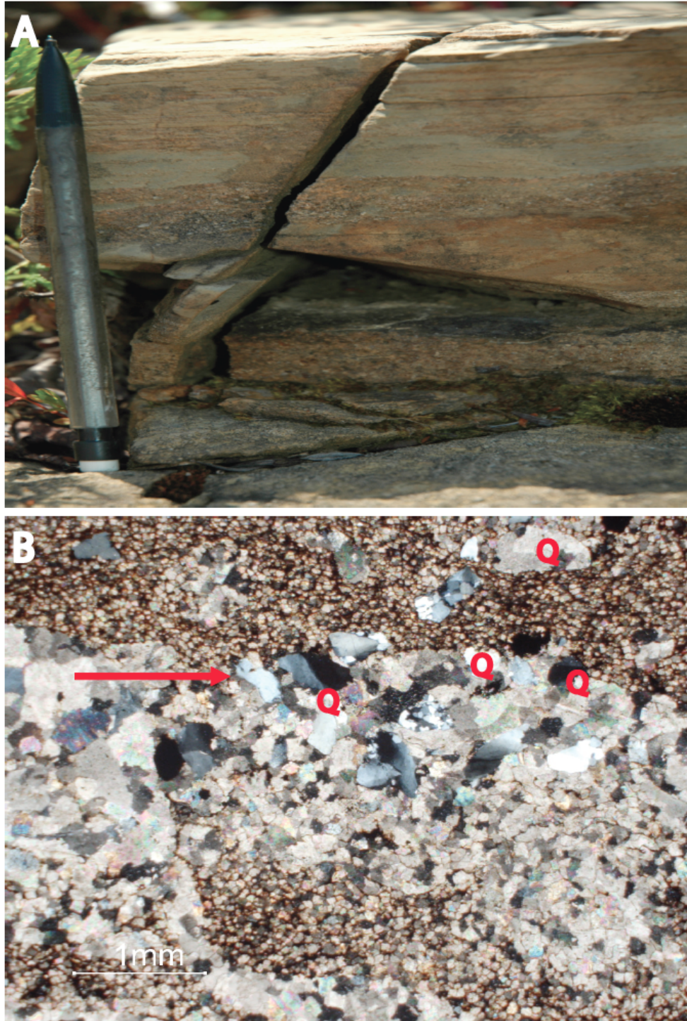
Figure 3.20: A) Field photo exhibiting the contact between the upper crinoidal dolostone unit and siltstone of the shale-mudstone unit. B) Contact between dolostone and siltstone in thin section (indicated by arrow). Q, quartz grains. Photo (A) courtesy of P.L. Corcoran.
