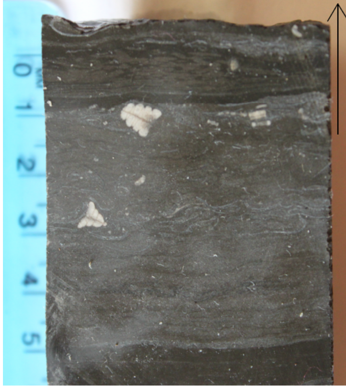
Figure 3.24: Oblique cut views of Ordovician crinoid stems found in the wackestone-packstone unit in Imperial #644 core.
