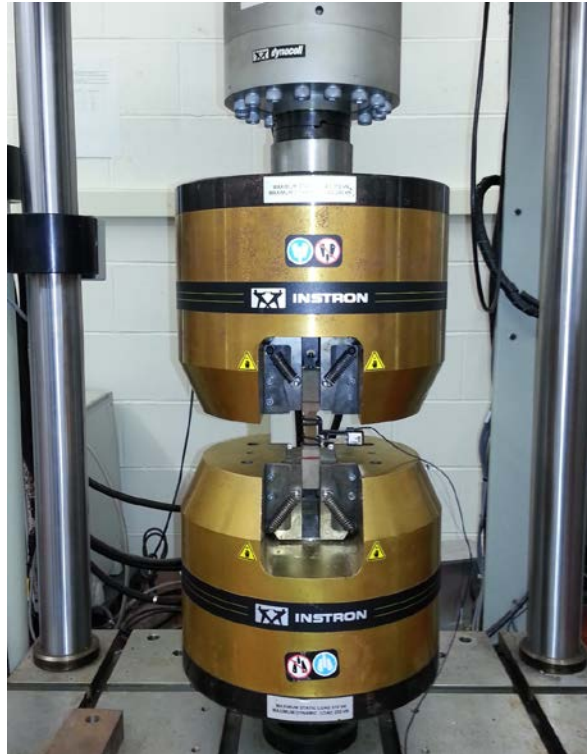
Figure 2.25: Cyclic test set-up of RPF sample
