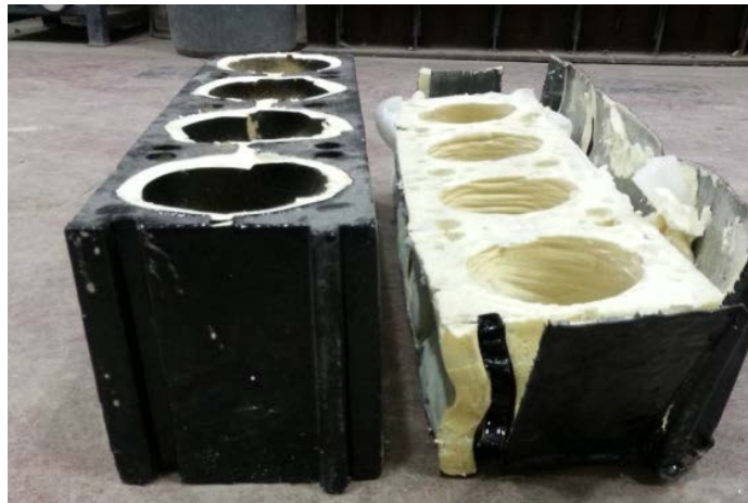
Figure 2.16: Poly-block before and after compression test
