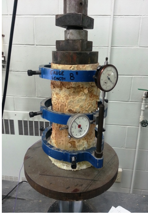
Figure 2.9: Poisson ratio test set-up
