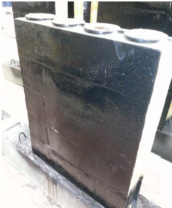
Figure 5.12: Wall inflation due to excessive heat
