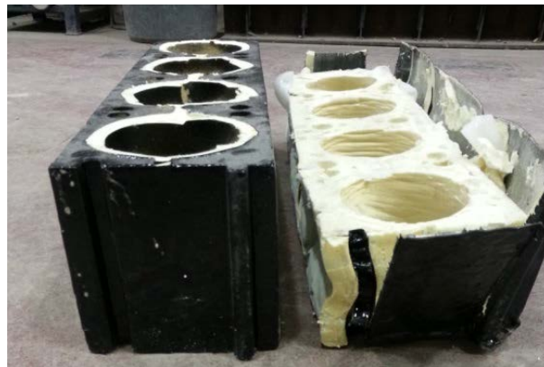
Figure 3.6: Poly-block experimental model before and after compression test
