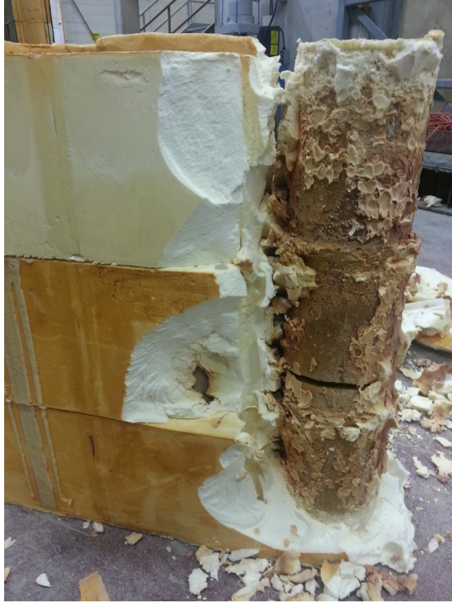
Figure 5.8: Crack in wall cores due to a pause in injection
