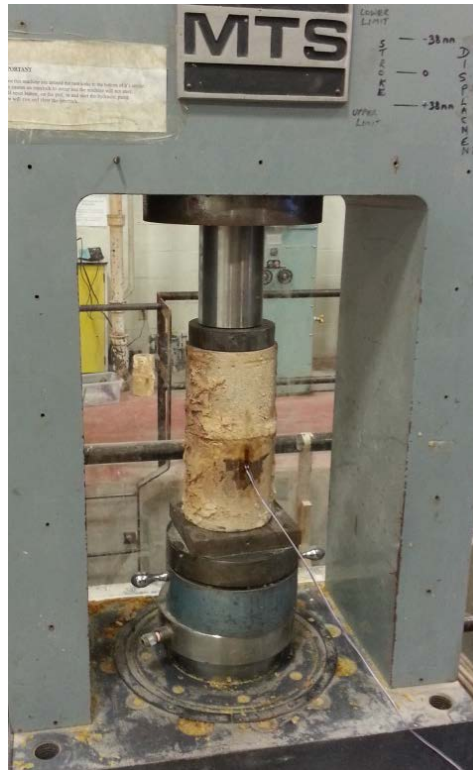
Figure 2.6: Compression test set-up
