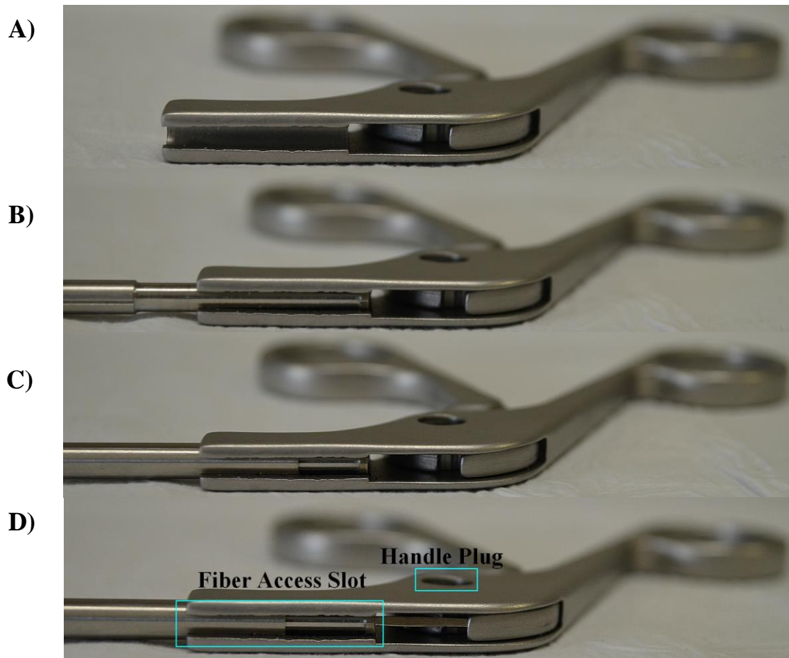
Figure 3.14: Grasper assembly view (a) handles; (b) sensor shaft; (c) outer shaft; (d) actuating rod.
