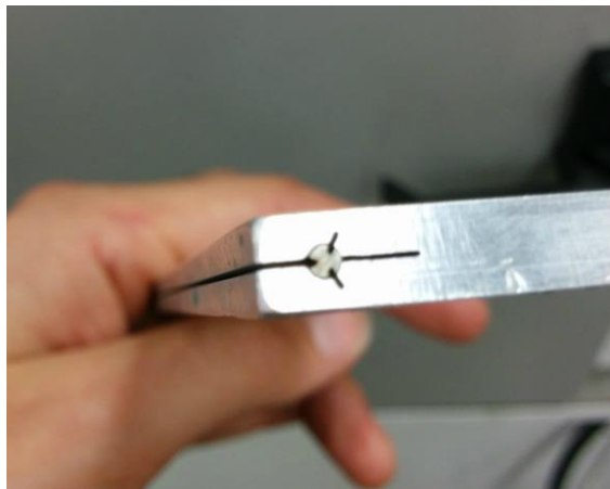
Figure 3.20: Probe clamp (a) EDM setup; (b) final grooves.
