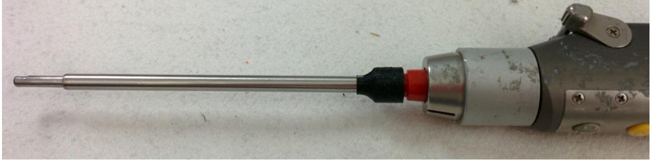
Figure 3.19: Shaver mounted in motor
