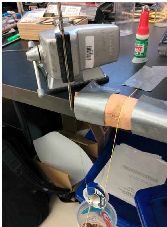
Figure 5.3: FBG pre-straining apparatus.
