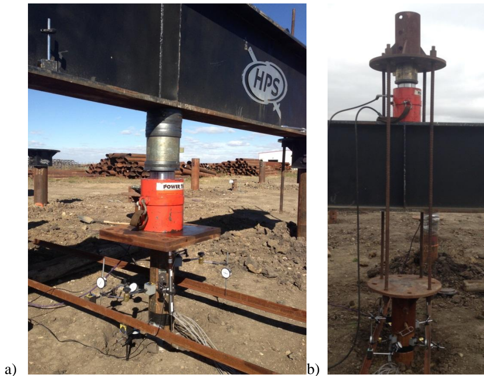
Figure 5-1: Loading Setup a) Compression b) Tension
