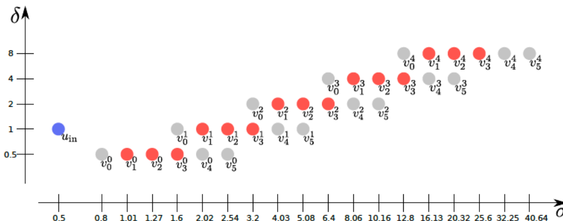
Figure 4.2: A representation of a standard scale space where each dot represents an interval image v_s^o Where o is the image's octave and s is the interval. The dots in red represent the images covering the whole octave while the dots in grey are used in extrema detection.
