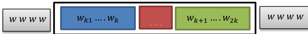
Figure 6: Inkpen's unsupervised method models the context as a window of k words before and after the near-synonym gap.
