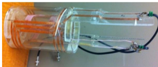
Figure 2-6: Transmit only/receive only saddle RF coil tuned to 0.883 MHz ( ^{129}\text{Xe} ) or 3.163 MHz ( ^1\text{H} ).
