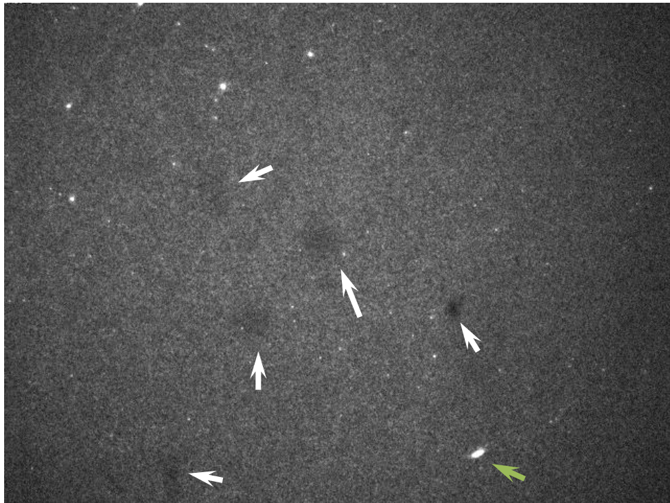
Figure 1.9: A sample frame from an image intensified camera. Dark portions related to dirt on the camera enclosure are marked with white arrows, while a meteor is marked with a green arrow. The mean brightness of the frame varies with distance to the edge, an example of vignetting. To compensate for these artefacts, the image is flat-fielded (procedure is discussed in Chapter 2).
