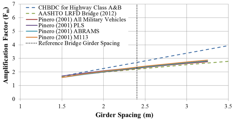
Figure 5.10 – Amplification factor versus girder spacing: Pre-Stressed Concrete Bridge (Pinero, 2001), 37 m CPCI girder bridge (Morrison Hershfield Ltd., 2012)
