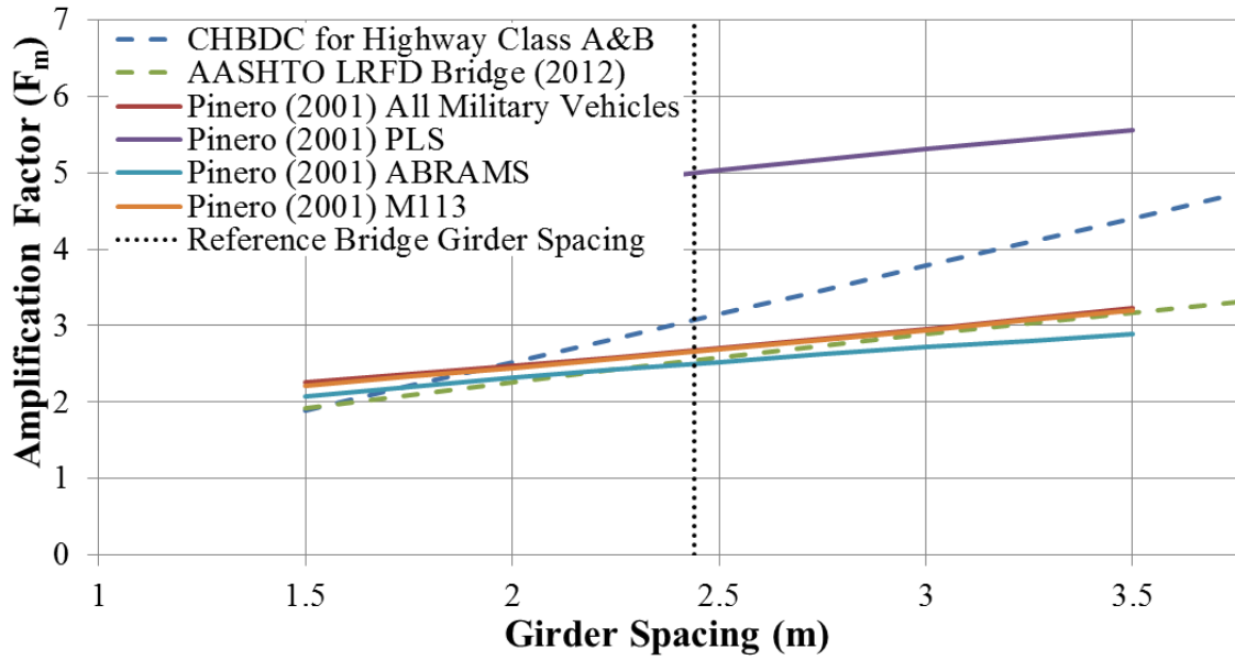
Figure F.3 - Amplification factor versus girder spacing: Steel Girder Bridges (Pinero, 2001), 36 m steel girder bridge (Kim, Tanovic, & Wight, 2010)
