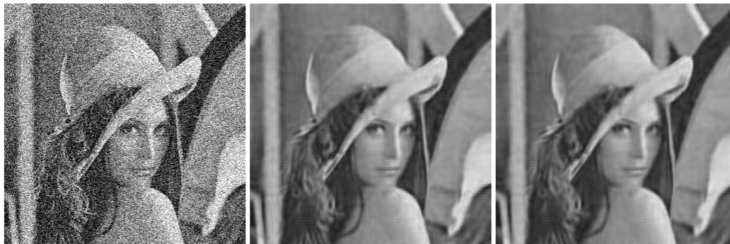
Figure 4.14: Subjective Comparison of DC-Only Profile with 50% Overlapping. Left: Noisy Image, Middle: BM3D Output, Right: Proposed Method's Output.
