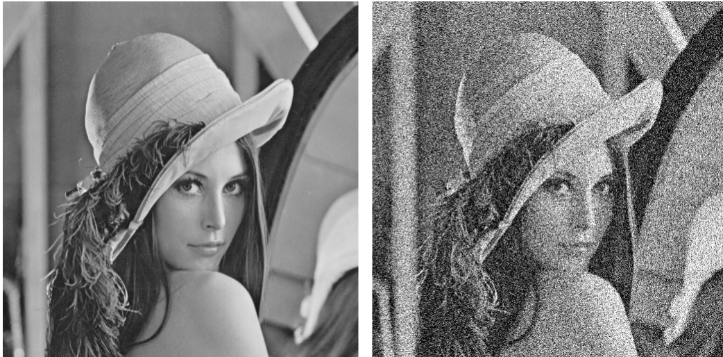
Figure 2.2: Example of Additive White Gaussian Noise. Left: Original Lena Image. Right: AWGN Added with Zero Mean and 0.05 Variance.
