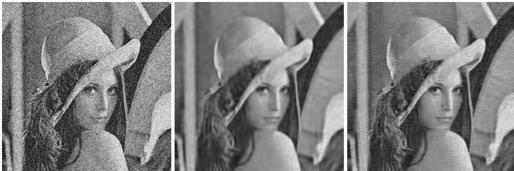
Figure 4.23: Subjective Comparison of DC-Only Profile with 75% Overlapping. Left: Noisy Image, Middle: BM3D Output, Right: Proposed Method's Output.
