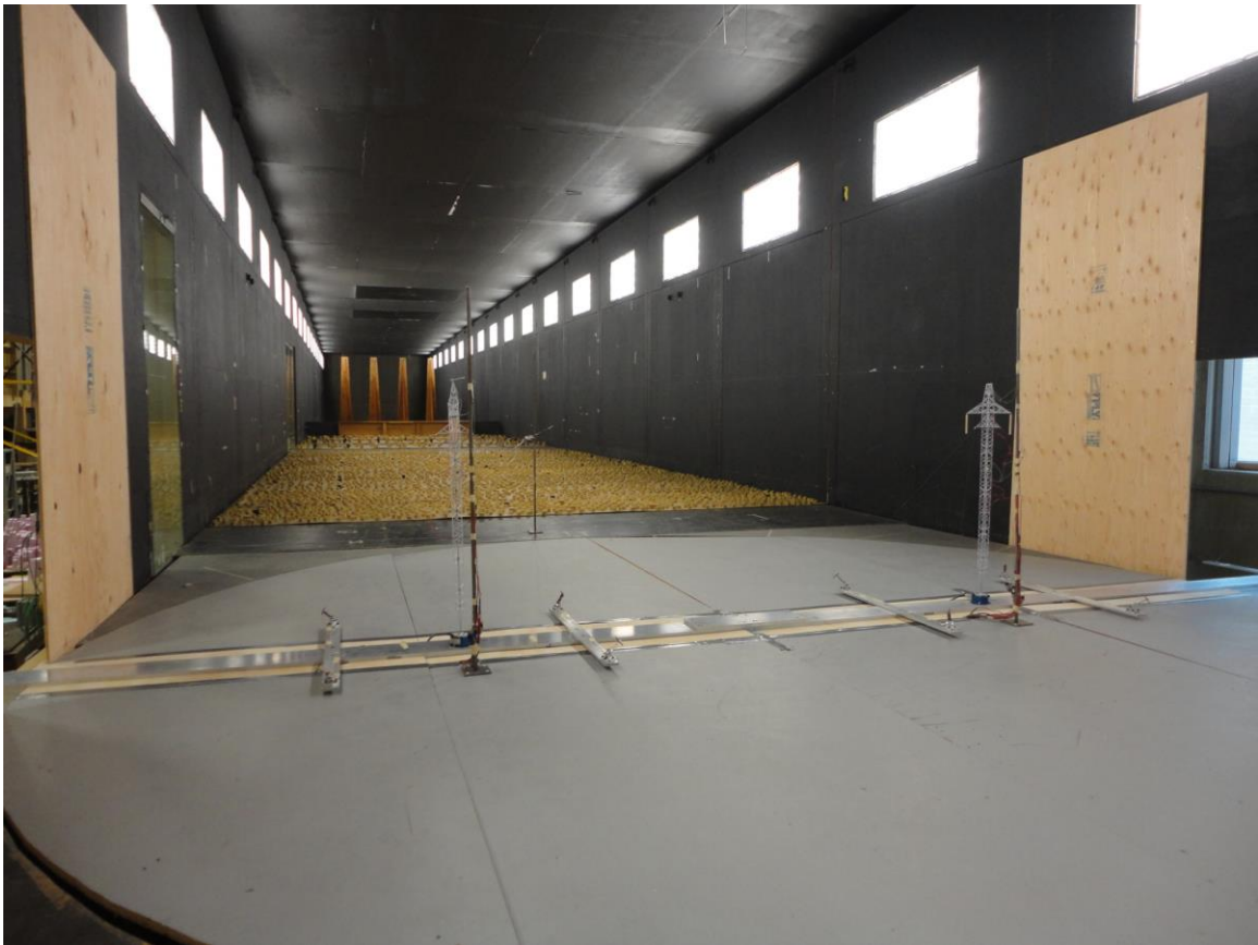
Fig. 6-13 Assembled Aeroelastic Transmission Line Model ( \Psi = 90^\circ )
