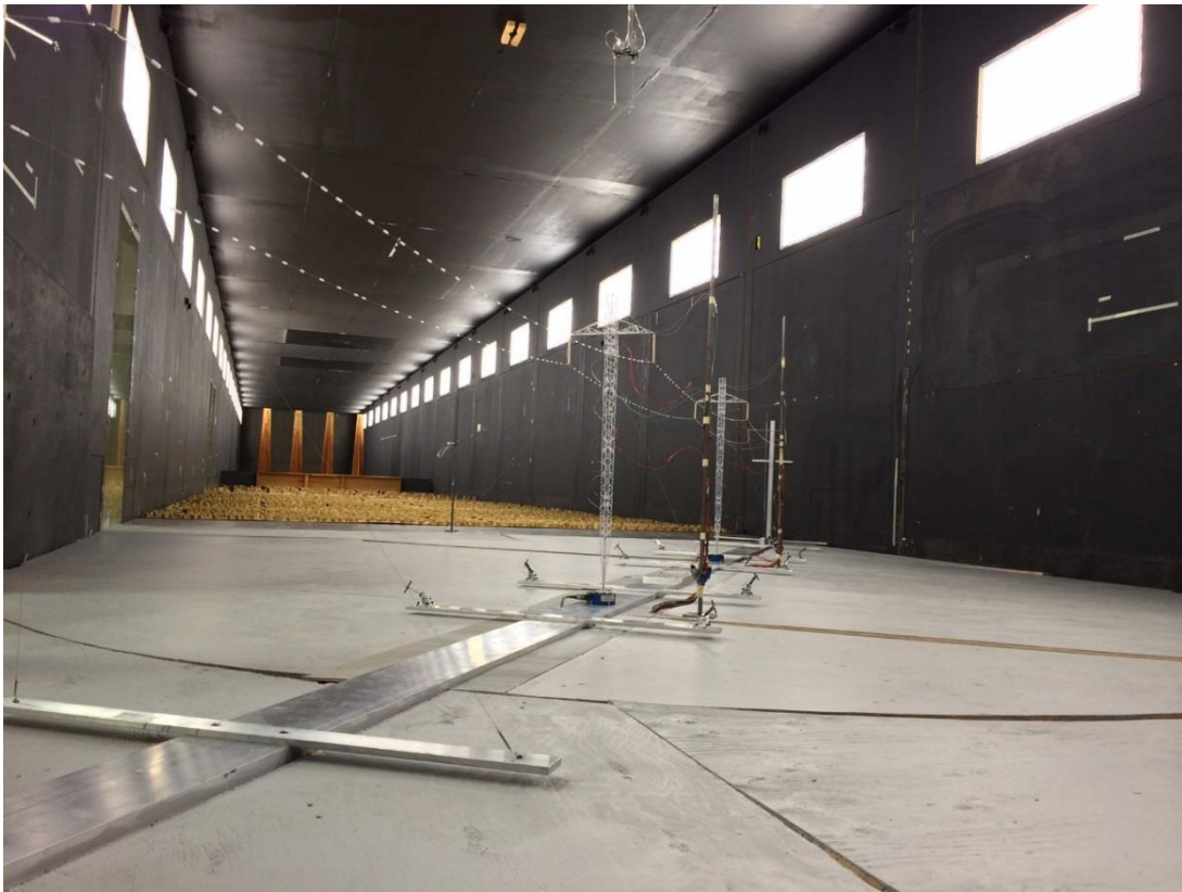
Fig. 6-4 Assembled Aeroelastic Transmission Line Model ( \Psi = 30^\circ )
