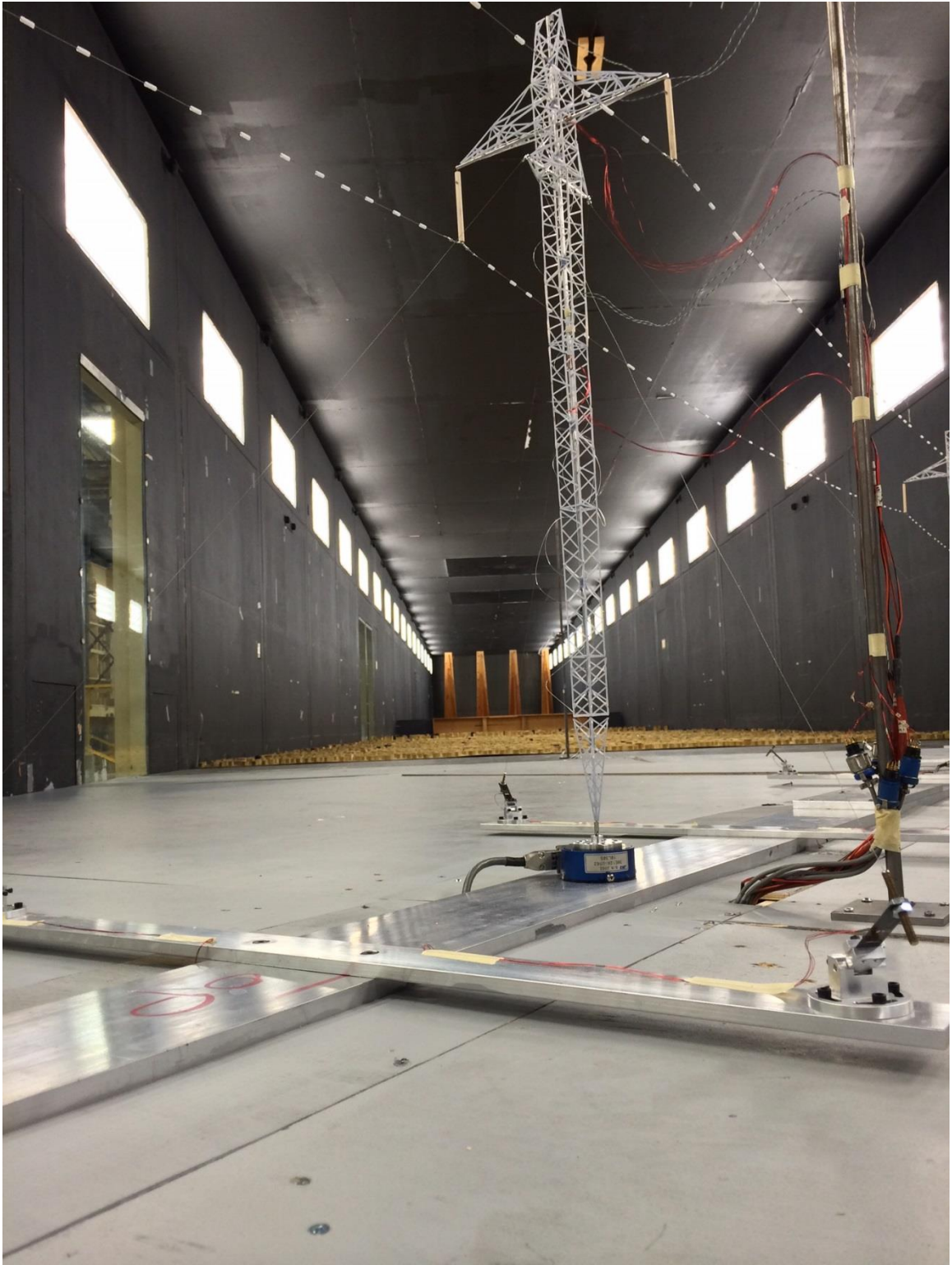
Fig. 6-8 Assembled Transmission Tower Aeroelastic Model
