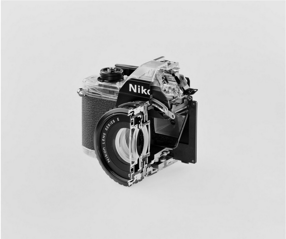
Figure 8. Christopher Williams, Cutaway model Nikon Em . Shutter: Electronically governed Seiko metal blade shutter, vertical travel with speeds from 1/1000 to 1 second, with a manual speed of 1/90th. Meter: Center-weighted Silicon Photo Diode, ASA 25-1600, EV 2-18 [with ASA film and 1.8 lens]. Aperture Priority automatic exposure. Lens Mount: Nikon F mount, Al coupling [and later] only. Flash: Synchronization at 1/90 via hot shoe. Flash automation with Nikon SB-E or SB-10 flash units. Focusing: K type focusing screen, not user interchangeable, with 3mm diagonal split image rangefinder. Batteries: Two PX-76 or equivalent. Dimensions: 5.3" x 3.38" x 2.13" [135mm x 86mm x 54mm], 16.2 oz [460g]. Fotostudio Axel Gnad, Düsseldorf October 17, 2008 [b&w], 2009. Gelatin silver print, 20 x 24 in. (50.8 x 61 cm).
