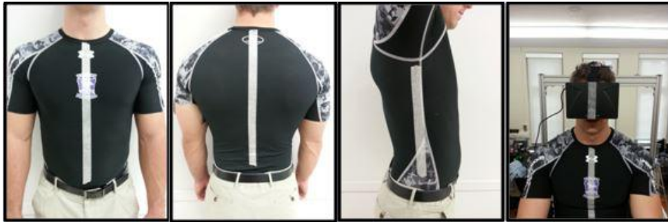
Figure 5: Images showing the strips of tape attached on the body of participant, and on the head-mounted display, for providing cues to help identify the operator's postures during the video analysis.
