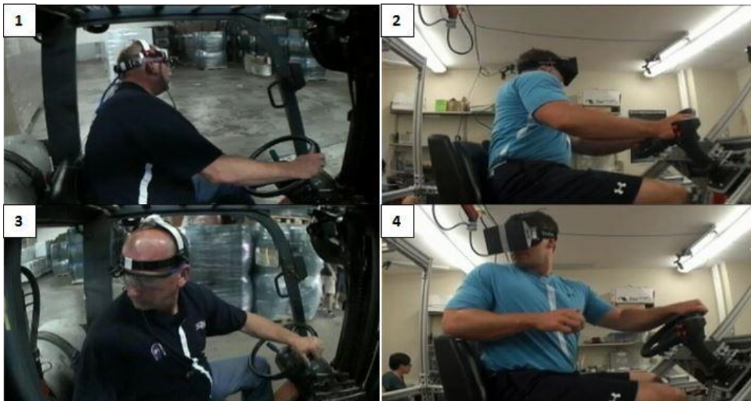
Figure 8: Illustration of the postures adopted by certified forklift operators in the field (1 & 3) and laboratory (2 & 4) for driving forward in the warehouse with a load (1 & 2) and driving backward in the warehouse unloaded (3 & 4).
