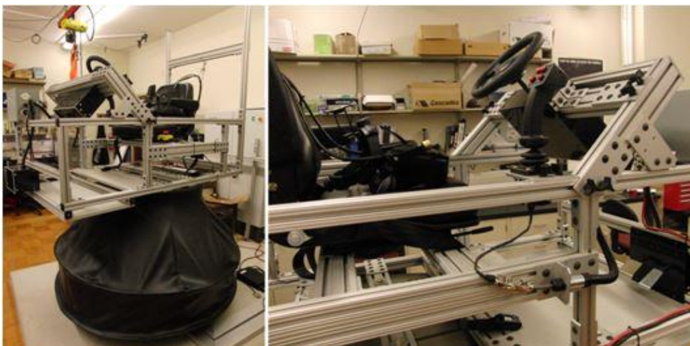
Figure 1: Custom designed cart (aluminum frame) mounted on the parallel robot (under the black skirt at the bottom of the left image). The vehicle controls (steering wheel, joystick, accelerator and brake pedals) are shown in the right image. Reproduced through Open Access from Dickey et al., 2013.
