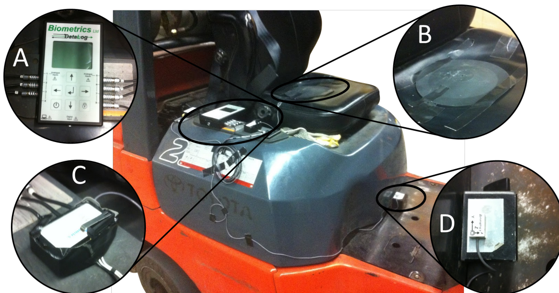
Figure 7: Data acquisition set-up for recording forklift vibrations including: A) DataLOG recording unit, B) seat pan form with embedded accelerometer, C) mechanical event marker, D) chassis accelerometer with magnetic mount.
