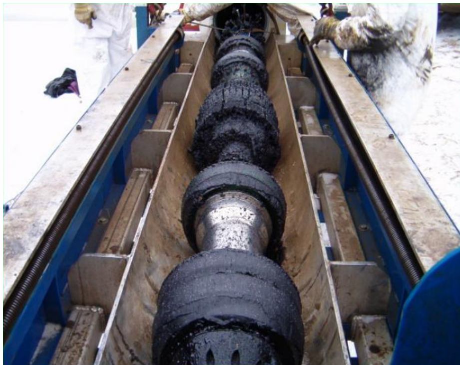
Figure 1.2 An ILI tool being retrieved from the pipeline after the inspection
