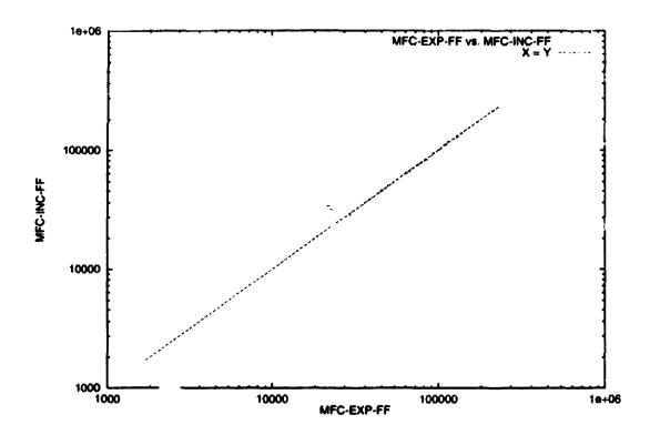
Figure 6.4: The number of constraint checks performed by MFC-EXP-FF versus the number of constraint checks performed by MFC-INC-FF on the same problem using the local model for problems with  $n=25,\ m=9$  and  $p_1\in\{0.2,0.25,\ldots,0.5\}.$  (350 problems).
