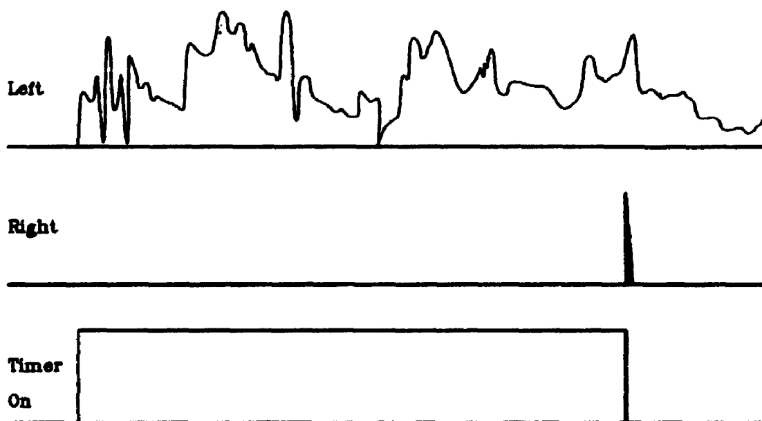
Figure F.1. Set-up of apparatus to measure tape speed. The left channel (stimulus onset) starts the timer; the right channel (trigger signal) stops the timer. In this way multiple samples of tape playing time can be taken from each tape.
