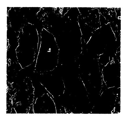
Figure 3.13: The edges extracted from the image shown in figure 3.8 after applying an adaptive threshold (i.e. the mode of the grey level frequency distribution, 16 in this case) to the edge strength.
