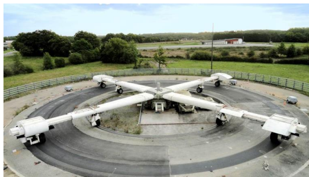
Figure 2: The IFSTTAR accelerated pavement testing facility
