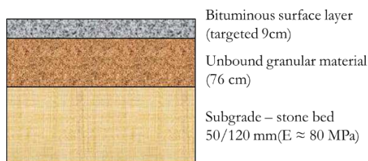
Figure 3: Tested pavement structures
