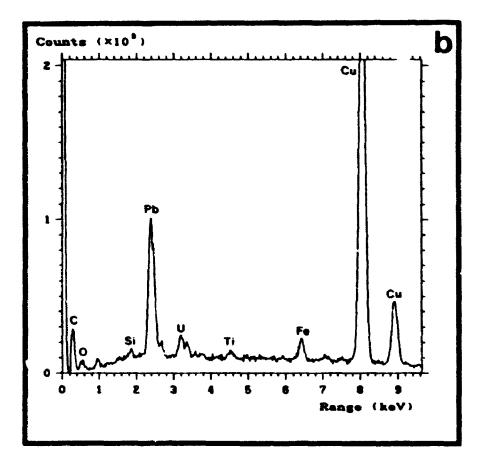
In the same samples, other cells showed the nucleation of small (approximately 100 nm in diameter), dense aggregates on the outer surfaces of the capsule (Plates 3 1b and 3.2a). Predominantly Fe-rich (Figure 3 2), these aggregates suggested an early stage of mineralization within the metal-loaded capsule, as represented in Plate 3 1a
