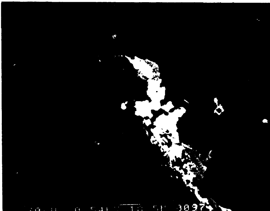
Plate 9 Scanning electron microscope image of baddelyite as fine-grained fracture filling within allanite, from lamprophyre dyke intersected in diamond drill hole B3839 at the NERCO-Con Mine.
