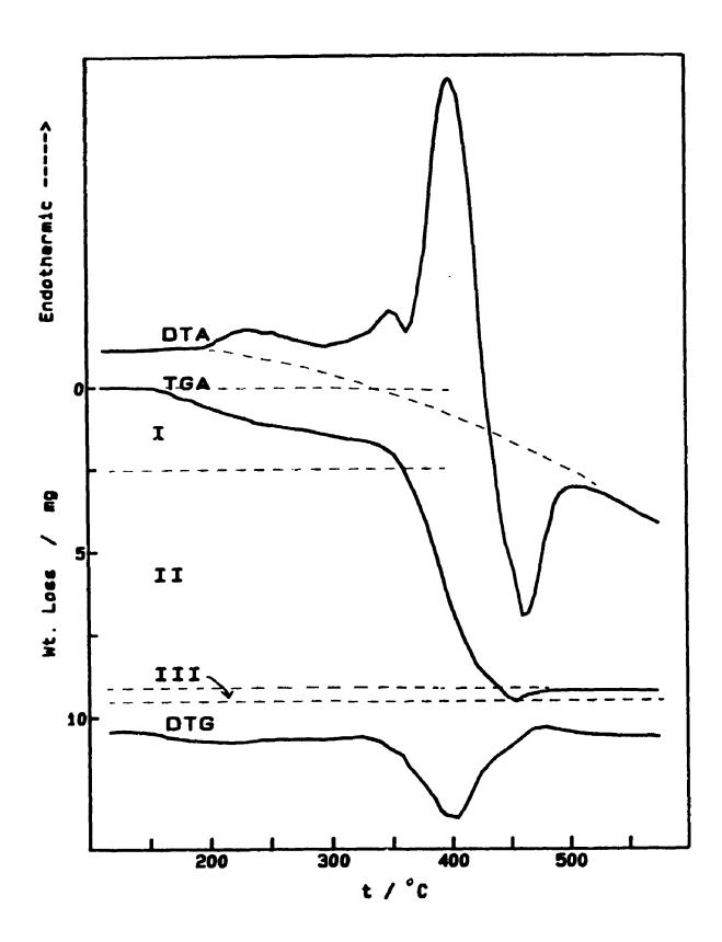
Fig. 6.3 TGA, DTA and DTG of cathodic deposits  $(NH_4)_4V_6O_{16}$  in air atmosphere. Scan rate 10 K/min. sample mass 103 mg.
