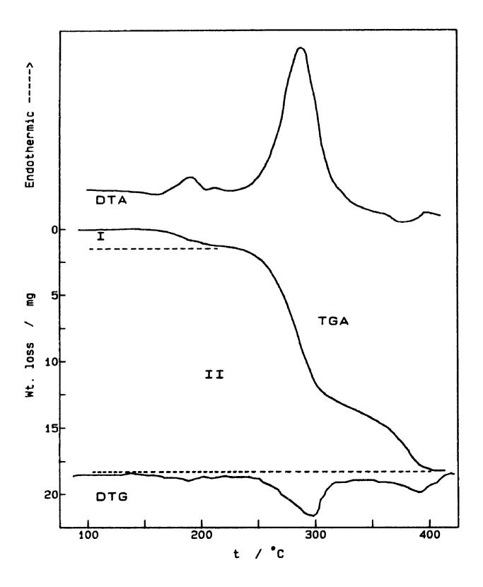
Fig. 6.5 TGA, DTA and DTG of cathodic deposits, of mixed phase  $(NH_4)_{0.9}K_{3.1}V_6O_{16}$  in argon atmosphere. Scan rate 10 K/min. sample mass 55 mg.
