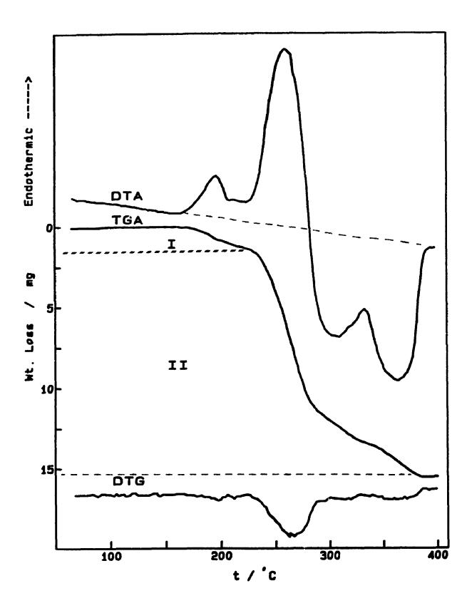
Fig. 6.4 TCA, DTA and DTG of cathodic deposits,  $(NH_4)_4V_6O_{16}$  in argon atmosphere. Scan rate 10 K/min. sample mass 100 mg.
