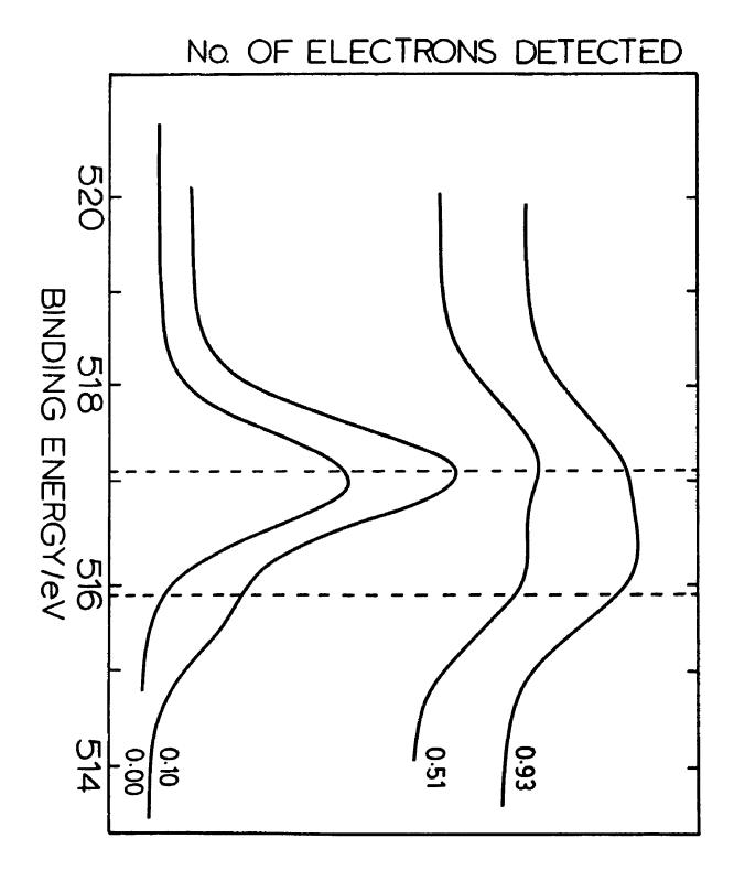
Fig. 6.8 Binding energies for V(IV), V(V), O(530), O(531) against x in Li  $_X$ V  $_2$ O  $_5$ .
