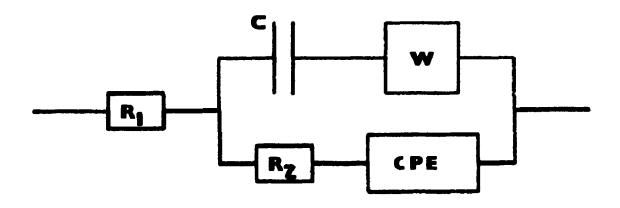
Table 8.2 Parameters of the equivalent circuit for impedance results as a function of the state of charge/discharge of the cell Li/tetraglyme-LiClO<sub>4</sub>/V<sub>2</sub>O<sub>5</sub>; T = 50°C.
