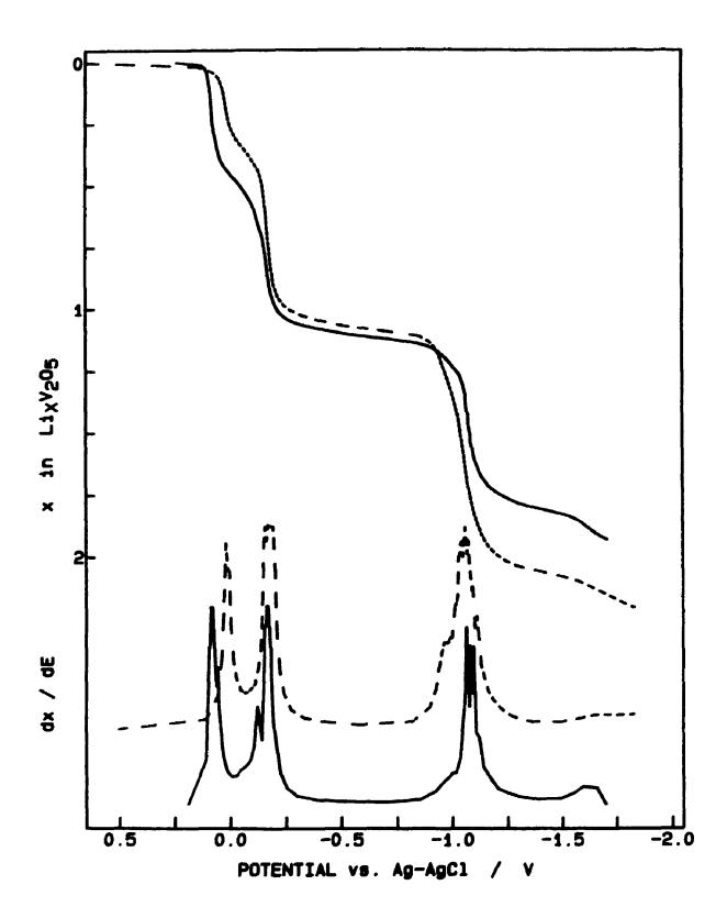
Fig. 6.10 Insertion and removal of lithium from  $V_2O_5$  electrode on Pt substrate at current density of  $0.2 \text{ mA/cm}^2$ , showing increasing hysterysis with increase in total insertion of Li. Max. x = 0.8 (——); max.  $x = 1.1(\cdots)$ : max. x = 1.45 (- - -).
