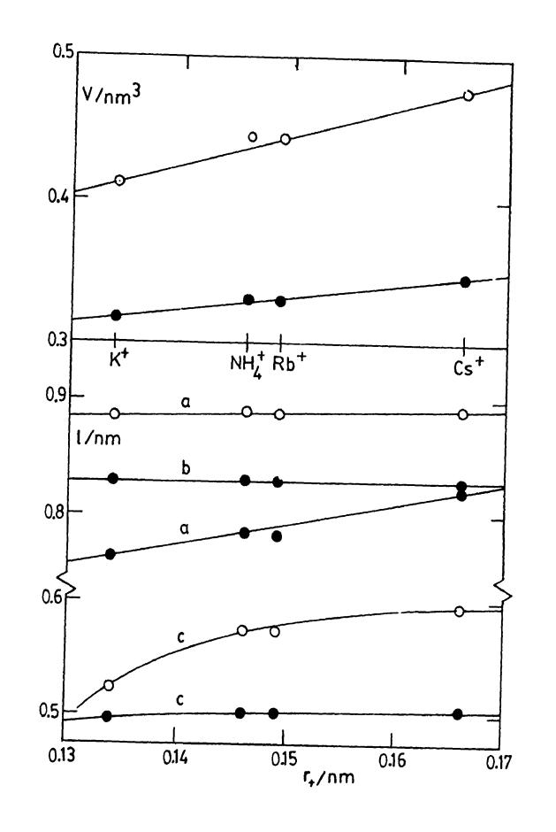
Fig. 5.4 Dependence of the lattice parameter I and volume V of unit cells in  $(NH_4)_XM_{4-X}V_6O_{16}$  on X for M-K (open circles), M-Cs (closed circles).
