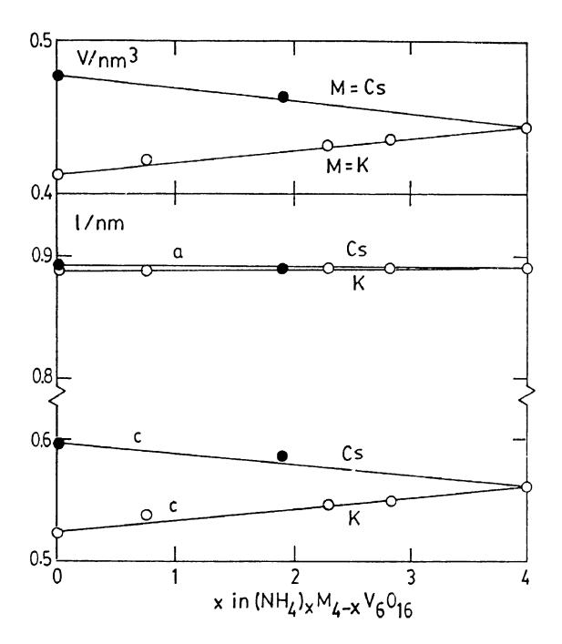
Fig. 5.5 Compositions of homogeneous phases in the quaternary system  $K_2O = (NH_4)_2O = V_2O_4 = V_2O_5$ .  $a, a' = (NH_4)_2V_6O_{16}, K_2V_6O_{16}; b, b' = (NH_4)_4V_6O_{16}, K_4V_6O_{16}$  [59];  $c = V_3O_7; d = 3K_2O \cdot 5V_2O_5 \cdot V_2O_4; e = K_2V_8O_{17}; f = K_2V_6O_{13}; g = K_4V_3O_7; h, h' = NH_4VO_3 KVO_3; j = (NH_4)_2V_3O_7.$  Solid area: results of [27]; diagonal hatching: results of [24]; vertical hatching: this thesis.
