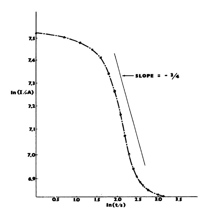
Fig. 7.4 Q - function for diammonium hexavanadate  $(\cdots)$ , tetrammonium hexavanadate (---) and  $V_2O_5$  (thermally decomposed tetrammonium hexavanadate) (----).
