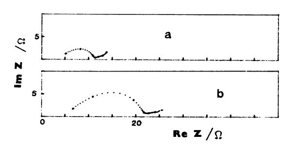
Fig. 8.5 Impedance spectrum as a function of the state of charge/discharge of the single cell battery.
