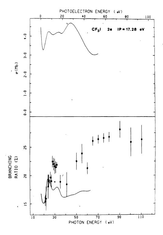
Experimental and theoretical MS-X $\alpha$  (solid lines) results , are shown for the photoionization of the 3a1 orbital of CF3I. The upper and bottom plots give the partial cross section  $\sigma$ , and branching ratio, respectively.
