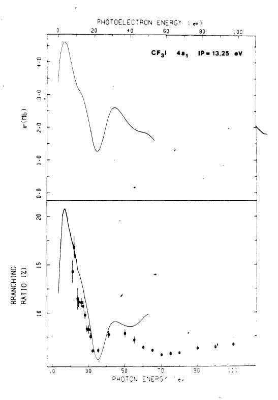
Experimental and theoretical MS-X $\alpha$  (solid lines) results are shown for the photoionization of the 3e and 1 $\grave{a}_2$  orbitals of CF3I. The upper and bottom plots give the partial cross section  $\sigma$ , and branching ratio, respectively.
