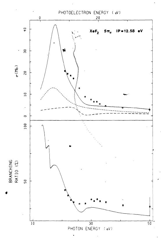
The upper plot shows the experimental and theoretical MS-X $\alpha$  (——) photoionization cross section (in Mb) of the  $40\sigma_g$  valence orbital of XeF2; plus the partial-channel cross sections for  $10\sigma_g \rightarrow k\sigma_u$  (——) and  $10\sigma_g \rightarrow k\pi_u$  (····). The bottom plot gives the theoretical MS-X $\alpha$  (——) and experimental branching ratios.
