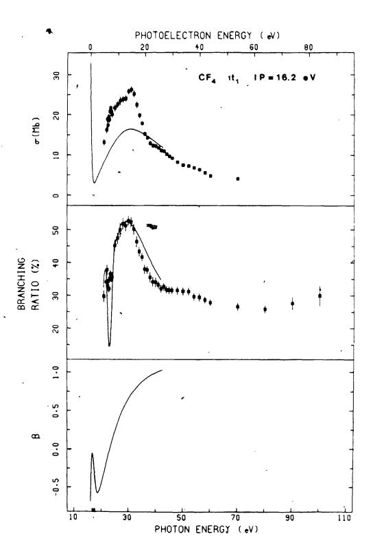
Experimental and theoretical MS-X $\alpha$  (solid lines) results on the photoionization of the 4t<sub>2</sub> orbital of CF<sub>4</sub>. For a direct comparison of our  $\sigma$  values with those of Carlson (Ref. 61), see Table 4.4.2-1. The upper, middle, and bottom plots give the  $\sigma$ , branching ratio, and  $\beta$  values, respectively.
