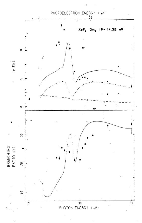
The upper plot shows the experimental and theoretical MS-X $\alpha$  (----) photoionization cross section (in Mb) of the  $4\pi_{\rm u}$  valence orbital of XeF<sub>2</sub>; plus the partial-channel cross sections for  $4\pi_{\rm u} \rightarrow {\rm k}\sigma_{\rm g}$  (---),  $4\pi_{\rm u} \rightarrow {\rm k}\pi_{\rm g}$  (····), and  $4\pi_{\rm u} \rightarrow {\rm k}\sigma_{\rm g}$  (----). The bottom plot gives the theoretical MS-X $\alpha$  (----) and experimental branching ratios.
