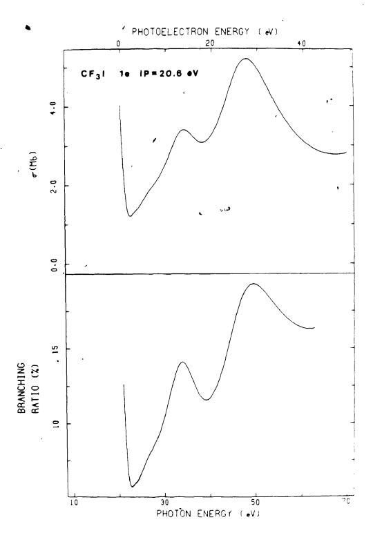
Theoretical MS-X $\alpha$  (solid lines) results are shown for the photoionization of the 2a<sub>1</sub> orbital of CF<sub>3</sub>I. The upper and bottom plots give the partial cross section  $\sigma$ , and theoretical branching ratio, respectively.
