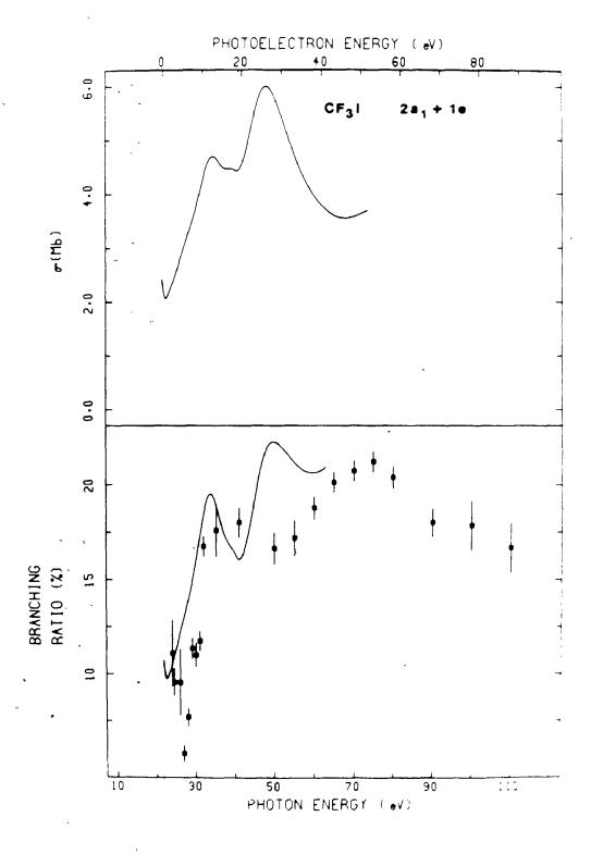
Theoretical MS-X $\alpha$  (solid lines) results are shown for the photoionization of the 1e orbital of CF<sub>3</sub>I. The upper and bottom plots give the partial cross section  $\sigma$ , and theoretical branching ratio, respectively.
