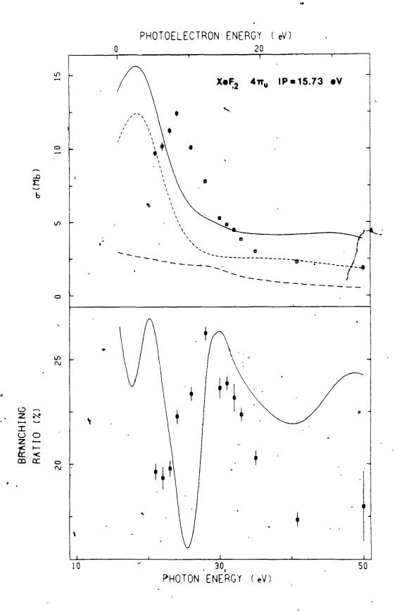
The upper plot shows the experimental and theoretical MS-X $\alpha$  (——) photoionization cross section (in Mb) of the  $6\sigma_u$  valence orbital of XeF2; plus the partial-channel cross sections for  $6\sigma_u \to k\sigma_g$  (——) and  $6\sigma_u \to k\pi_g$  (····). The bottom plot gives the theoretical MS-X $\alpha$  (——) and experimental branching ratios.
