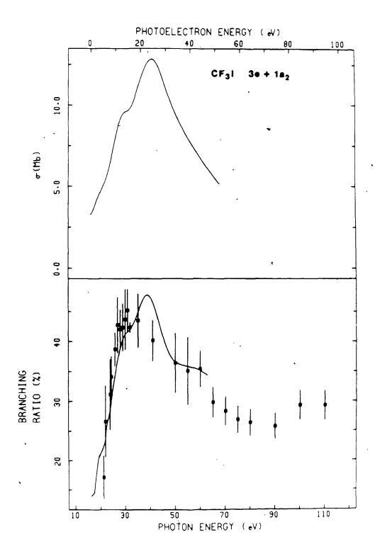
Theoretical MS-X $\alpha$  (solid lines) results are shown for the photoionization of the 1a2 orbital of CF3I. The upper and bottom plots give the partial cross section  $\sigma$ , and theoretical branching ratio, respectively.
