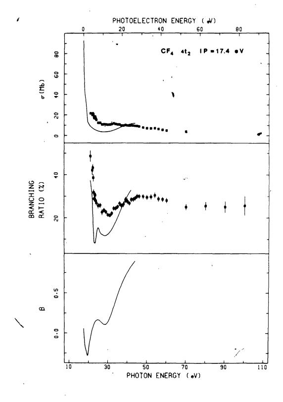
Experimental and theoretical MS-X $\alpha$  (solid lines) results on the photoionization of the 1 $\epsilon$  orbital of CF4. The upper, middle, and bottom plots give the  $\sigma$ , branching ratio, and  $\beta$  values, respectively.
