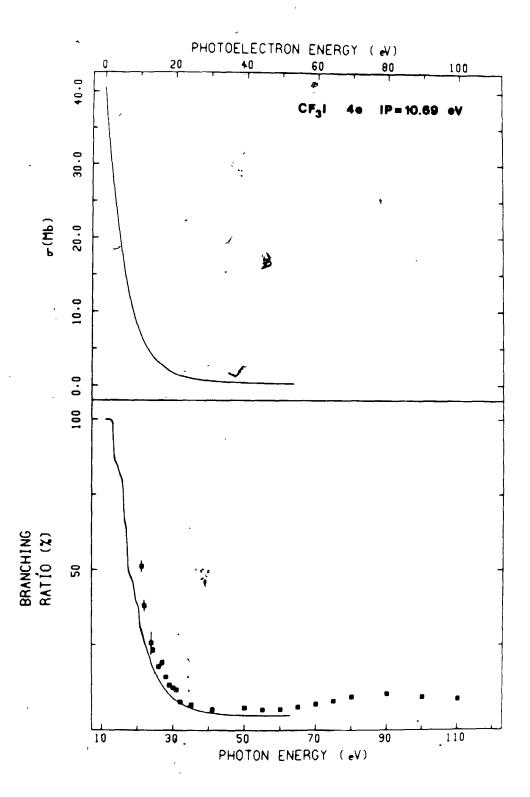
Experimental and theoretical MS-X $\alpha$  (solid lines) results are shown for the photogonization of the 4a<sub>1</sub> orbital of CP<sub>3</sub>I. The upper and bottom plots give the partial cross section  $\sigma$ , and branching ratio, respectively.
