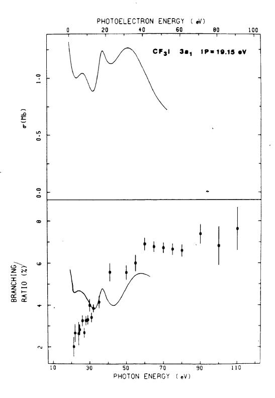
Experimental and theoretical MS-X $\alpha$  (solid lines) results are shown for the photoionization of the 2a<sub>1</sub> and 1e orbitals of CF<sub>3</sub>I. The upper and bottom plots give the partial cross section  $\sigma$ , and branching ratio, respectively.
