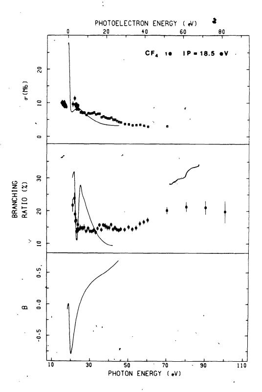
Experimental and theoretical MS-X $\alpha$  (solid lines) results on the photoionization of the 3t<sub>2</sub> orbital of CF<sub>4</sub>. The upper, middle, and bottom plots give the  $\sigma$ , branching ratio, and  $\beta$  values, respectively.
