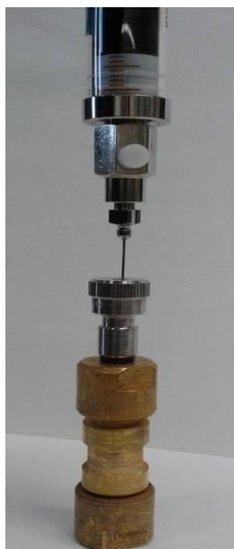
Figure 4.9: Sampling procedure using a leak-tight syringe.
