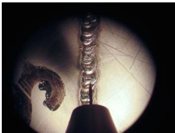
Figure 4.5: The view of Tungsten electrode tip fusing metal under microscope.
