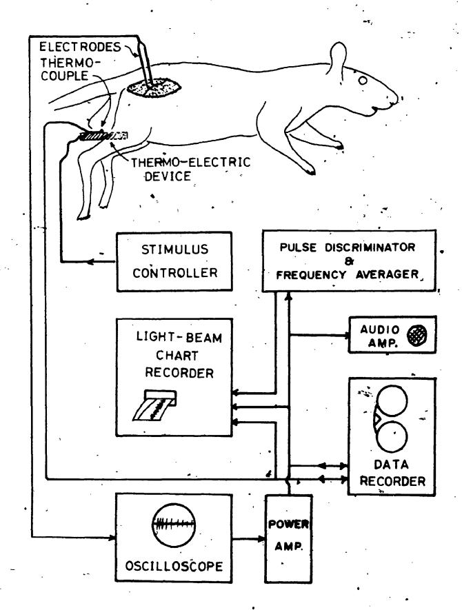
The final form of the data was a visual record made by a Honeywell Visicorder, Model 2106. This is the light beam chart recorder shown in Figure 4, and will commonly be referred to as "the Visicorder". In this recorder ultraviolet light is reflected from small galvanometers and focused on light sensitive paper to give a trace of the desired analogue signals. Up to 8 variables can be displayed on six inch paper with a single time grid using this recorder.
