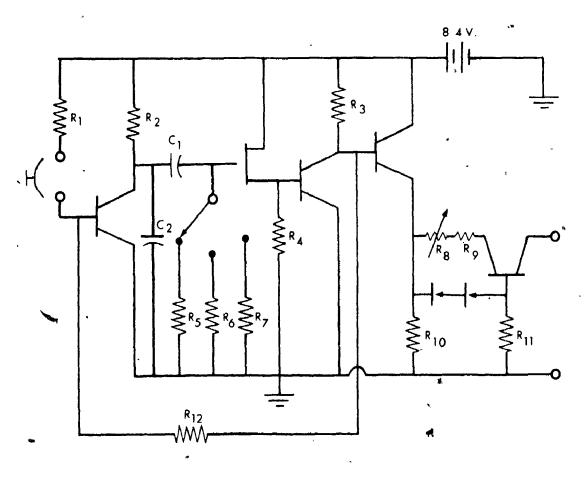
$R_{1} = -6.8 \text{ K}\Omega.$   $R_{2} = 10 \text{ K}\Omega.$   $R_{3} = 1 \text{ K}\Omega.$   $R_{4} = 1.5 \text{ K}\Omega.$   $R_{5} = 330 \text{ K}\Omega.$   $R_{5} = 660 \text{ K}\Omega.$   $R_{7} = 1 \text{ M}\Omega.$   $R_{8} = 2 \text{ M}\Omega.$   $R_{9} = 2 \text{ M}\Omega.$   $R_{10} = -90 \text{ K}\Omega.$   $R_{11} = 22 \text{ K}\Omega.$   $R_{12} = 10 \text{ K}\Omega.$
