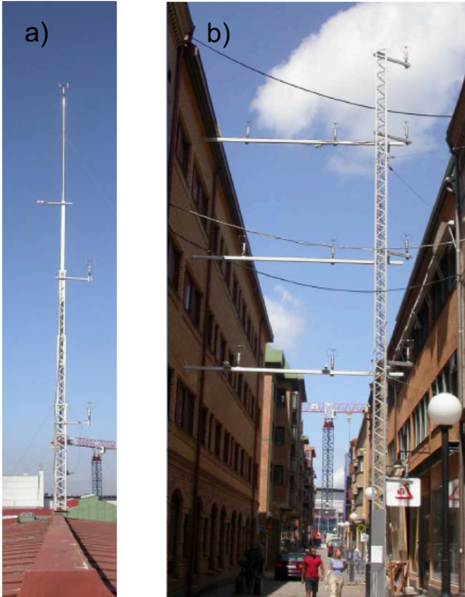
Figure 4 In-situ field study using sonic anemometers a) on building roof; b) within street canyon [4]
