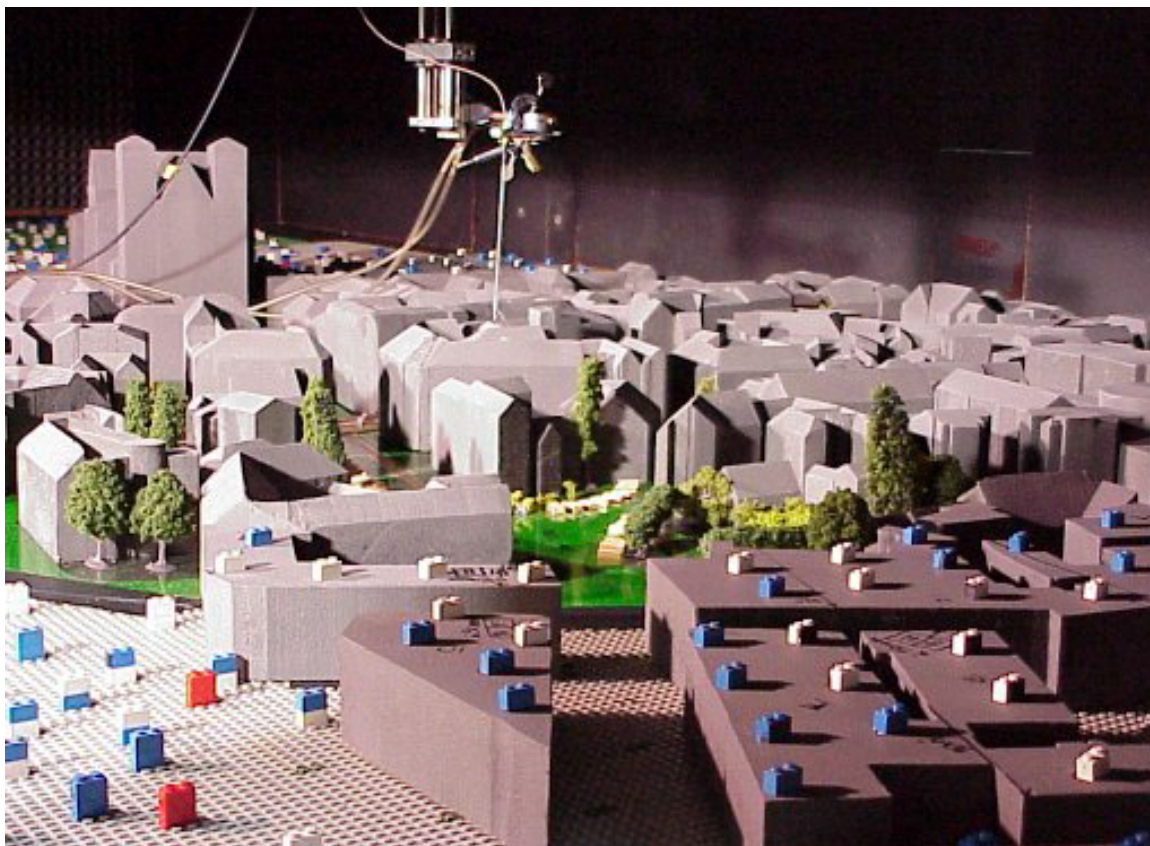
Figure 5 Site-specific wind tunnel model of ‘Rue de Strasbourg’ in Nantes and its surroundings [9]
