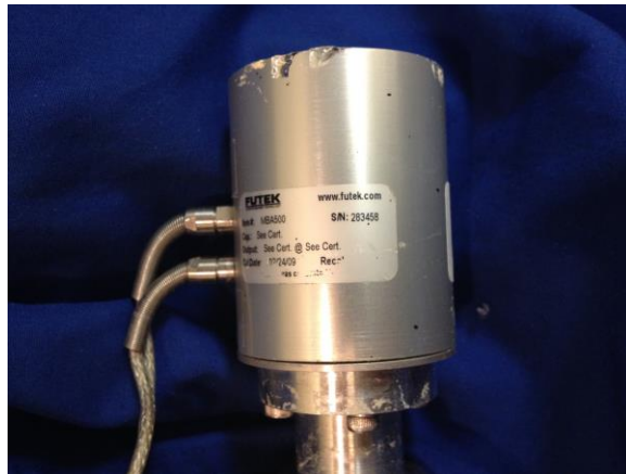
Appendix 4: Load Cell; capable of measuring axial loads as well as torque
