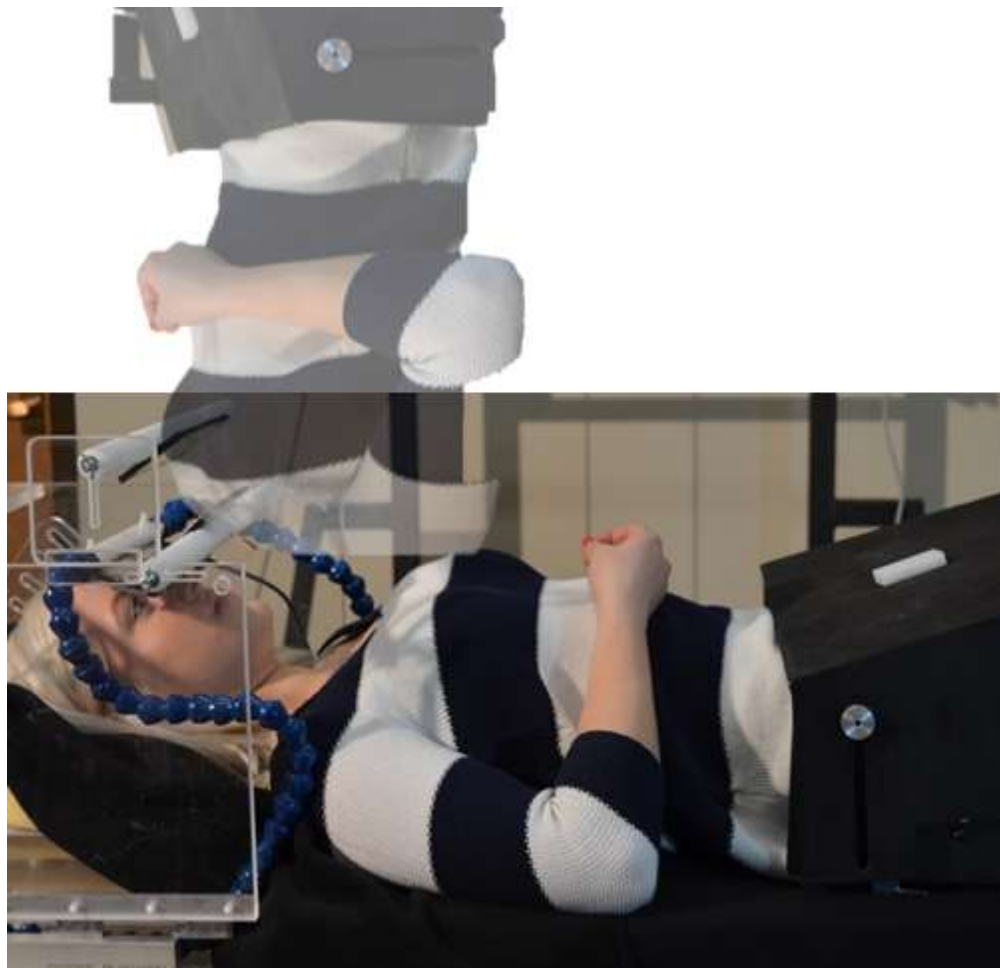
Figure 14. Due to the use of the mirror system used by many researchers participant receives conflicting visual cues and proprioceptive cues as to where their body exists in space during the indirect viewing condition. The participant sees their body as extending vertically but feels their body lying horizontal.
