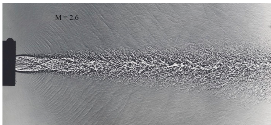
Figure 14. Shadowgraph of a Mach 2.6 cold jet. Jet oscillations cannot easily be observed in the initial part of the jet. Oscillation becomes visible at about ten jet diameters downstream of the nozzle exit. Oscillations extend to about 16 jet diameters before becoming blurred.
