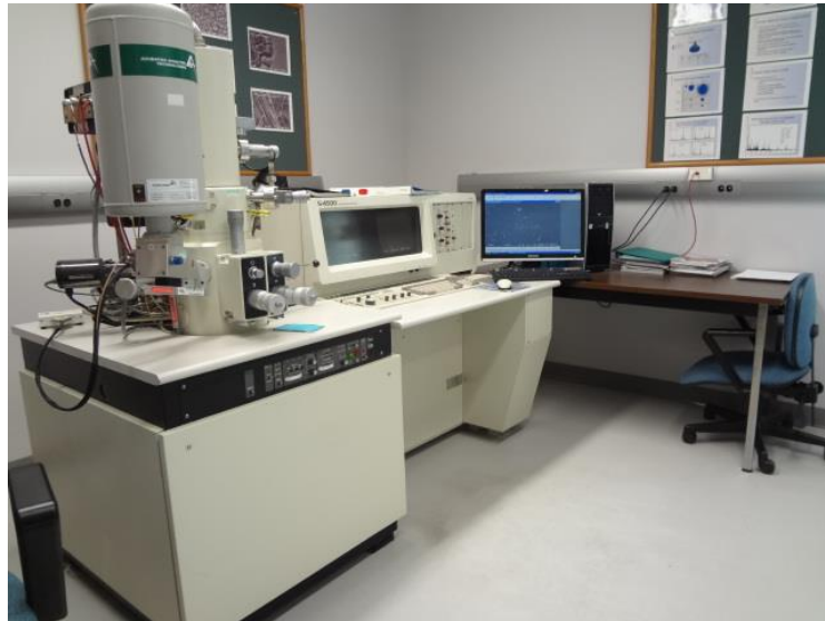
Figure 3.2: Illustration of SEM test apparatus.
