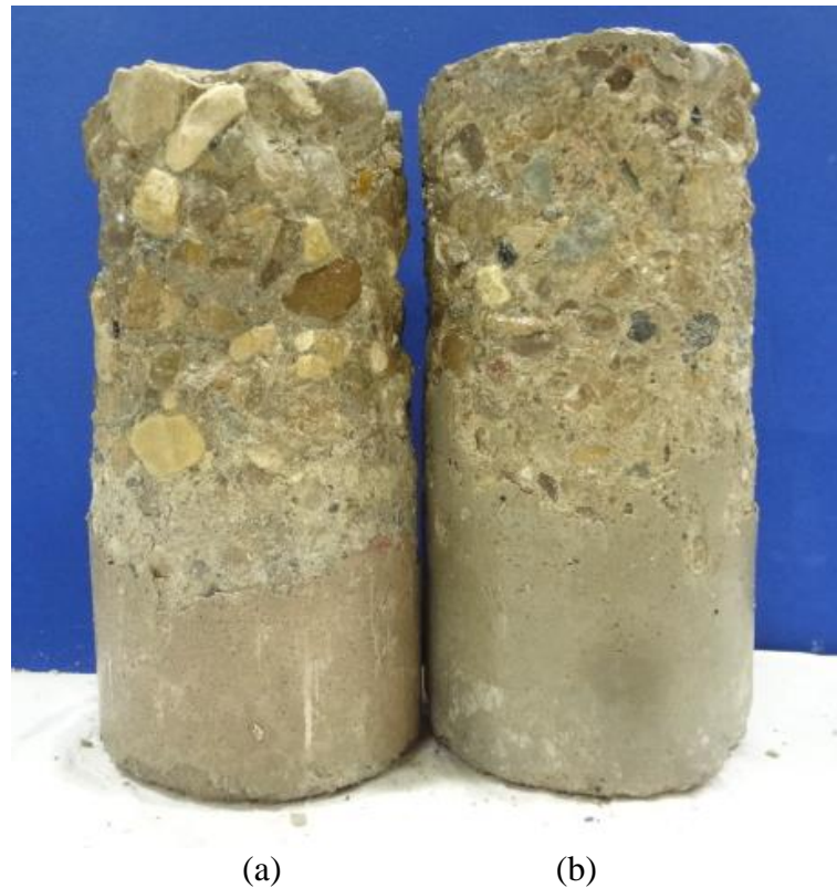
Figure 4.6: Effect of curing on physical sulphate attack of concrete made with OPC +25% FA at w/b = 0.60 : (a) non-cured specimen; and (b) specimen moist cured for 28 days.
