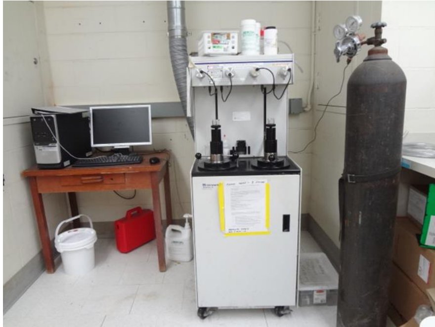
Figure 3.1: Illustration of MIP test apparatus.
