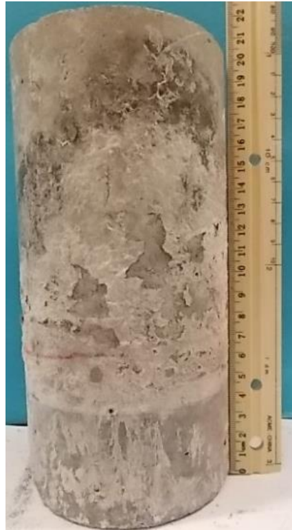
Figure 5.4: Damage of the acrylic layer of coated non-cured concrete made with w/b = 0.60 after two months of physical sulphate exposure.
