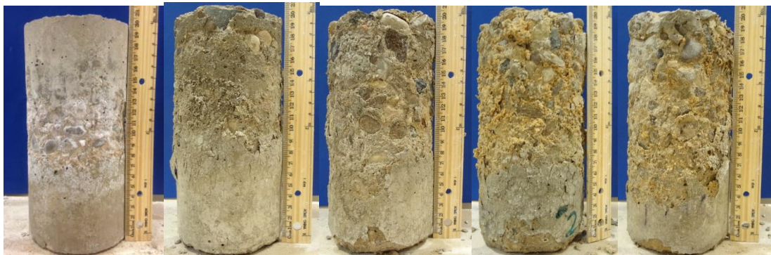
Figure 6.4: Damage due to salt crystallisation for concrete made with: (a) OPC; (b) OPC + 5% FA; (c) OPC + 10% FA; (d) OPC + 15% FA; and (e) OPC + 20% FA.
