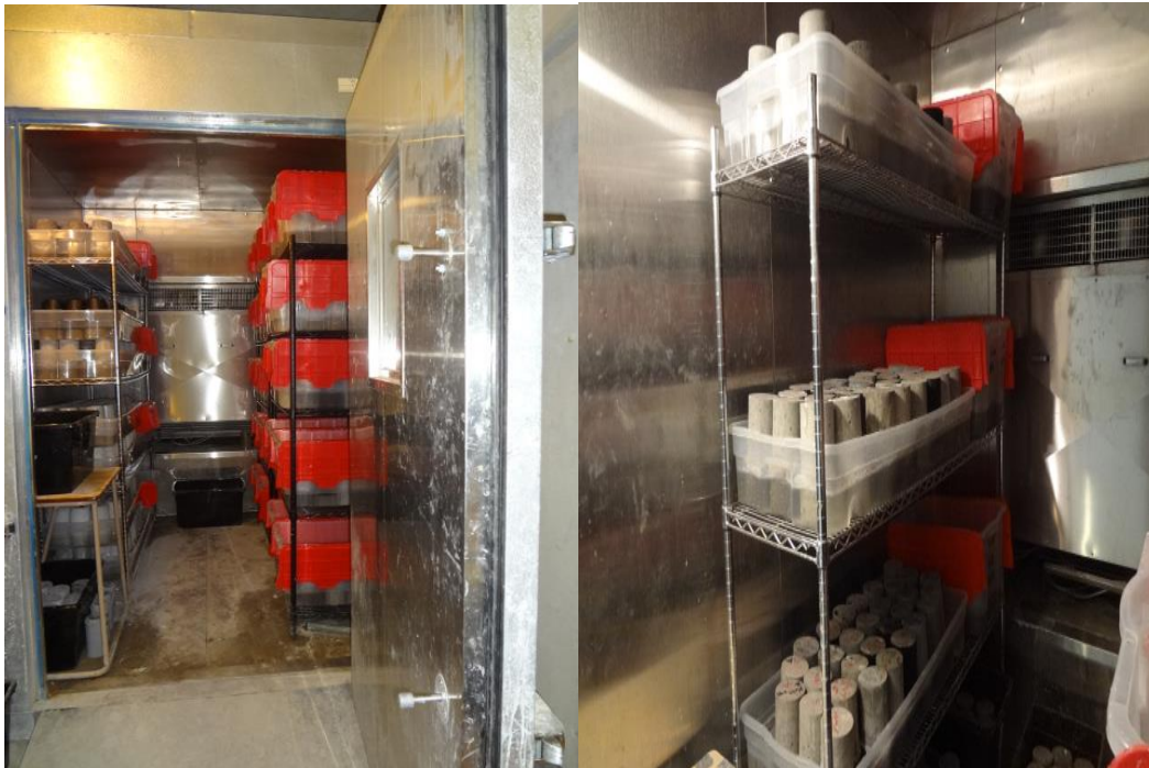
Figure 4.1: Tested specimens in the environmental chamber.
