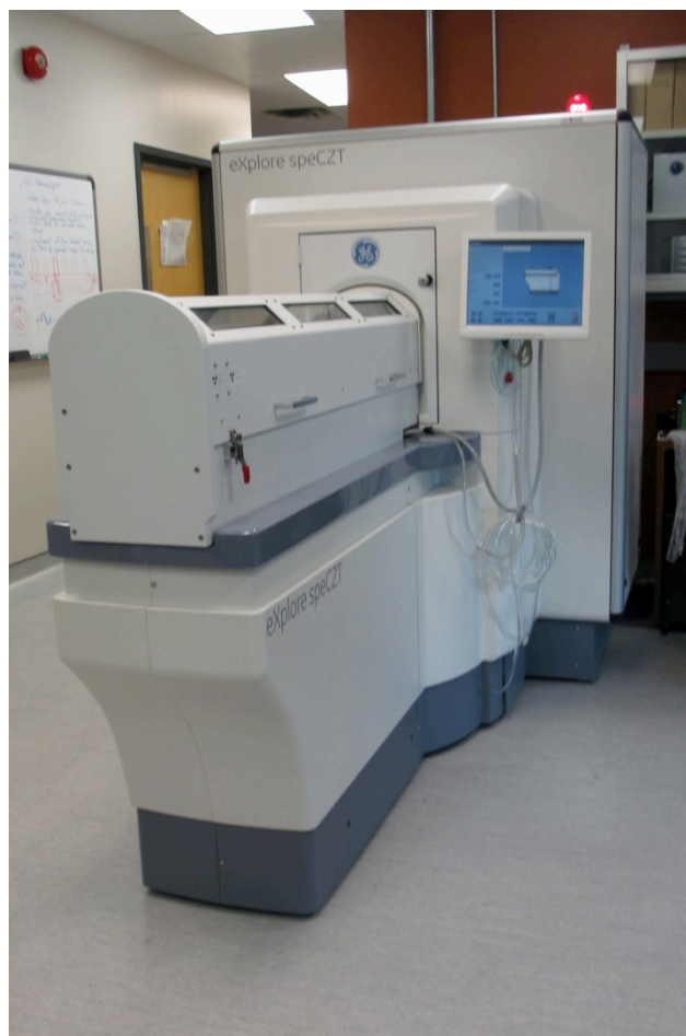
Figure 1.2 - GE eXplore speCZT. Located at the Robarts Research Institute, this scanner was utilized for both testing of beam hardening correction as well as collection of volumetric meteoritic data.
