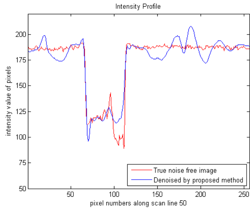
Figure 4-18: Intensity profile of House image and denoised image by proposed method at scan line 50 ( \sigma=100 )
