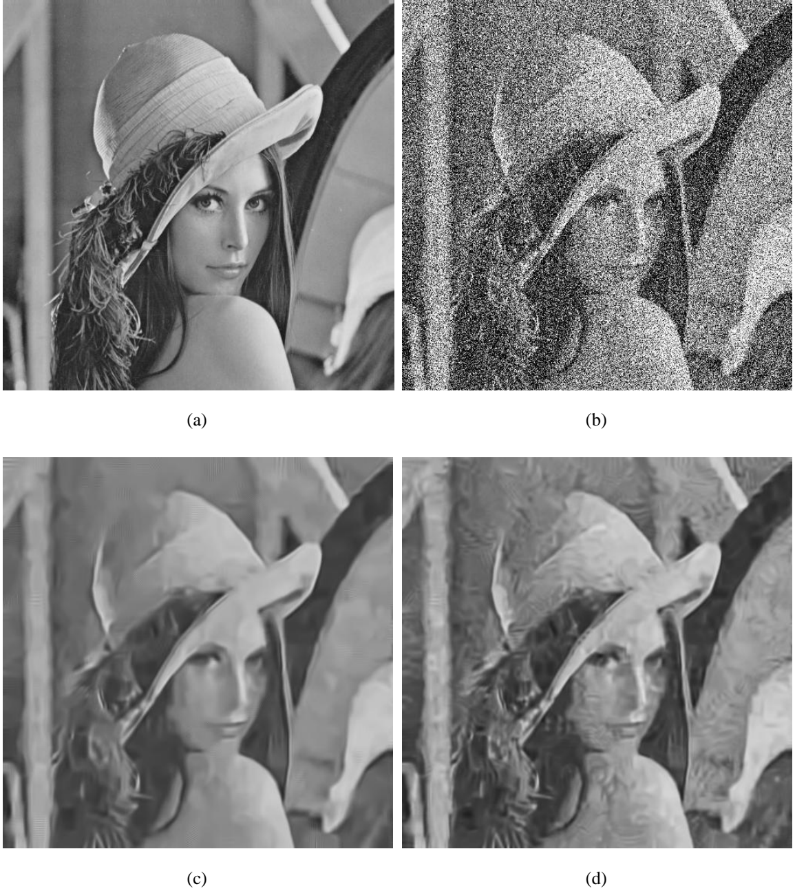
Figure C-13: Subjective comparison of denoising performance between BM3D and AEG-BM3D for standard test image Lena at noise level \sigma = 90 . (a) Noise free Lena image. (b) Noisy image with \sigma = 90 . (c) Denoised image using BM3D, PSNR = 24.5864, SSIM = 0.7259. (d) Denoised image using AEG-BM3D, PSNR = 25.3037, SSIM = 0.6933.
