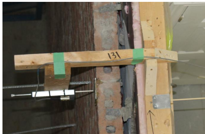
Figure 3.19 - LVDT WN5, measuring relative brick-top plate displacement
