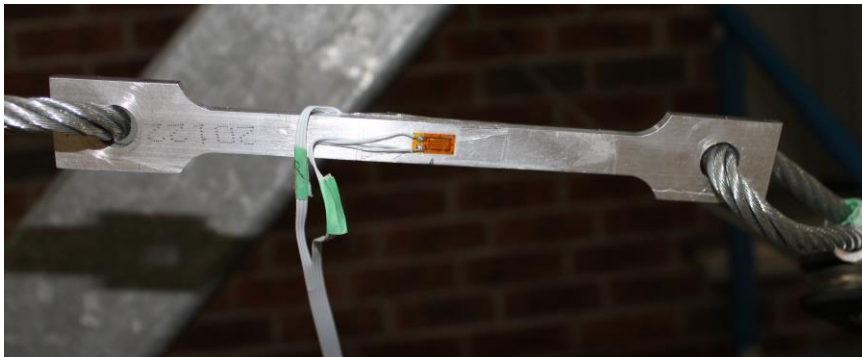
Figure 3.17 - Close up view of a strain gauge attached to an aluminum piece, forming a load cell.
