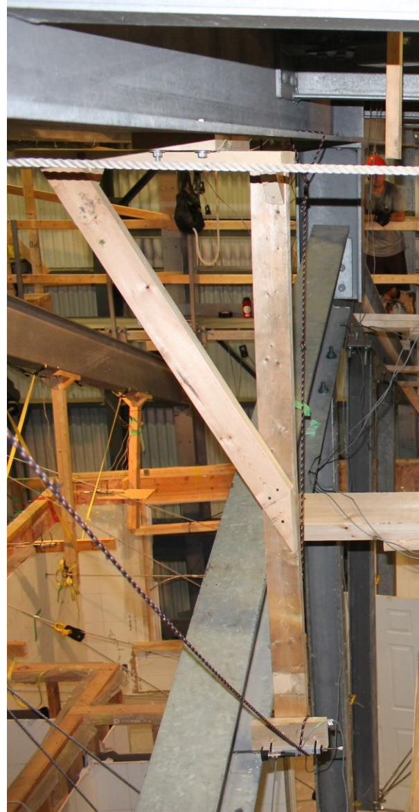
Figure E1 - LVDT dropping down from higher up on the reaction frame to record gable beam rotations.
