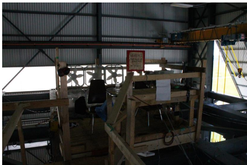
Figure 3.23 - The control platform on top of the reaction frame.
