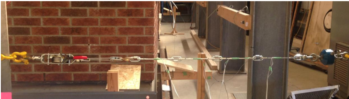
Figure F1 - Strain gauge calibration test setup. From left to right, come-along to apply load, three load cells and digital load cell.
