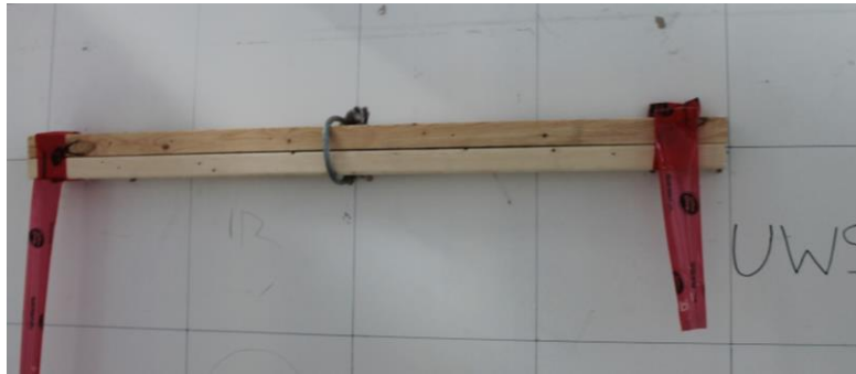
Figure 3.7 - A wood spreader beam installed at B10, on the second floor, set up to apply negative pressure (outwards loading).
