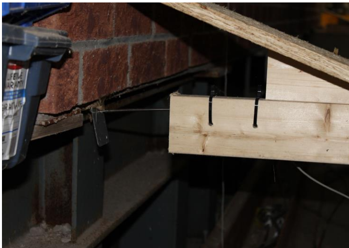
Figure A13 - Displacement Transducer North East 5
