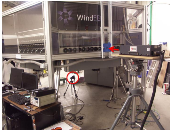
Figure 3-7: PIV setup for horizontal velocity field measurements in MWD.
