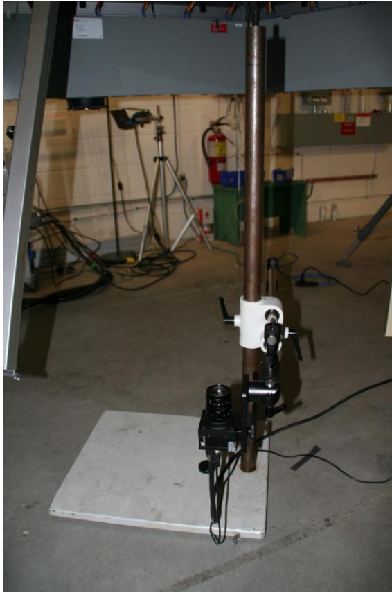
Figure 3-6: Camera setup for horizontal plane measurements.
