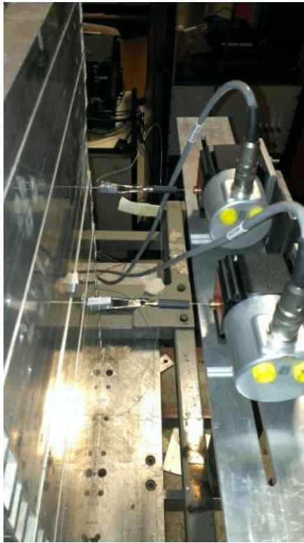
Figure 2-6: The Wire Line Position Sensors mounted on a frame and tied to the wires
