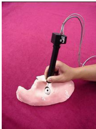
Figure 1.7: Micron, an active hand-held device for tremor cancellation [18] (Copyright © The Robotics Institute, Carnegie Mellon University)
