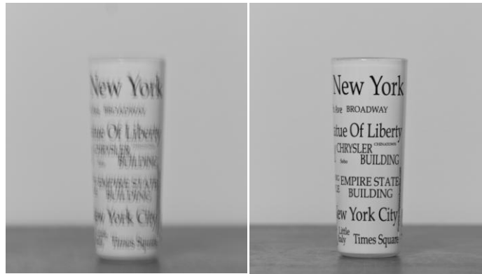
Figure 1.11: (Left) Image blur without image stabilization; (Right) Sharp image with image stabilization by Canon
