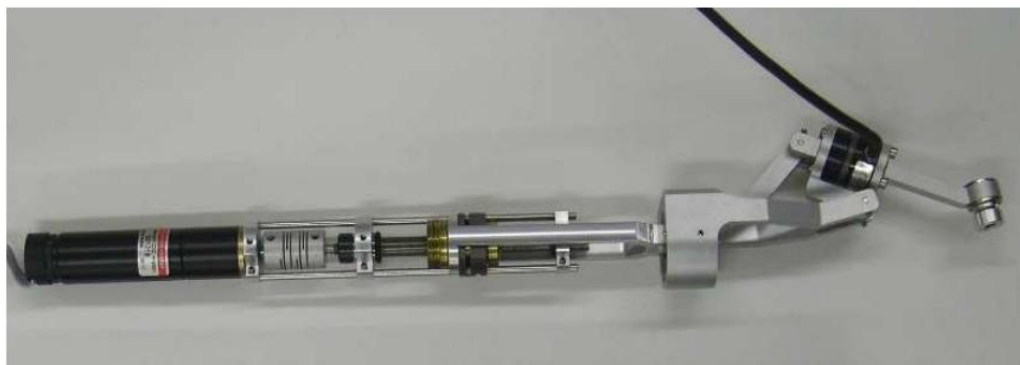
Figure 1.17: Tilt mechanism of the second prototype of SHR [52] (Copyright © 2007, IEEE)
