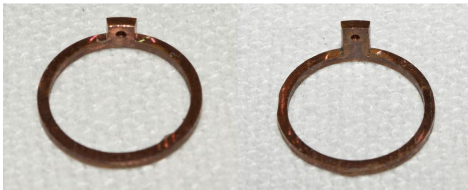
Figure 4.10: Electrodes that drive the IPMC actuator. (Left) Inner electrode (away from the needle tip); (Right) Outer electrode (near the needle tip)
