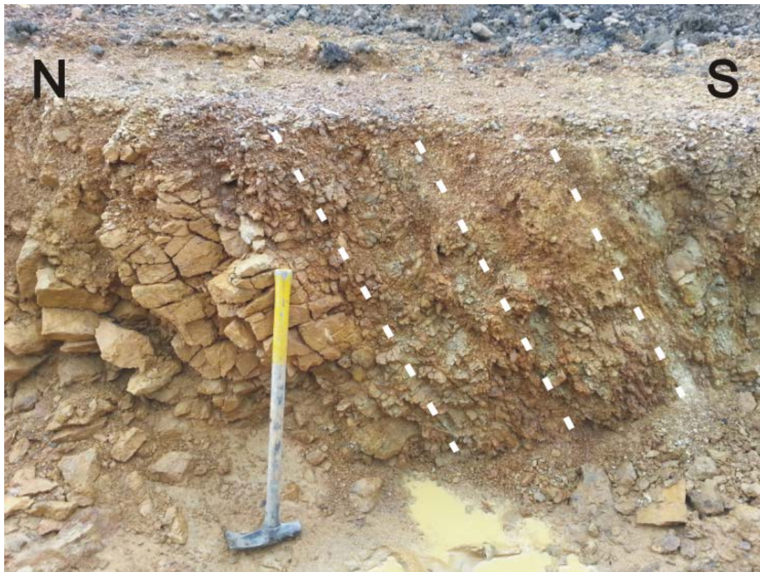
Figure 5.2: Surface expression of Latte mineralization. Looking east. A mineralized corridor dips SSW. Geotool for scale.
