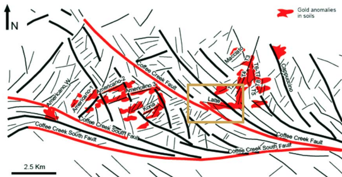
Figure 5.1: Local Coffee Creek fault array. The Latte fault splay is highlighted within the gold box. Note it is a splay off a 1 st order NW-trending fault, but not a regional shear zone (red). Modified after Sanchez et al., 2013.
