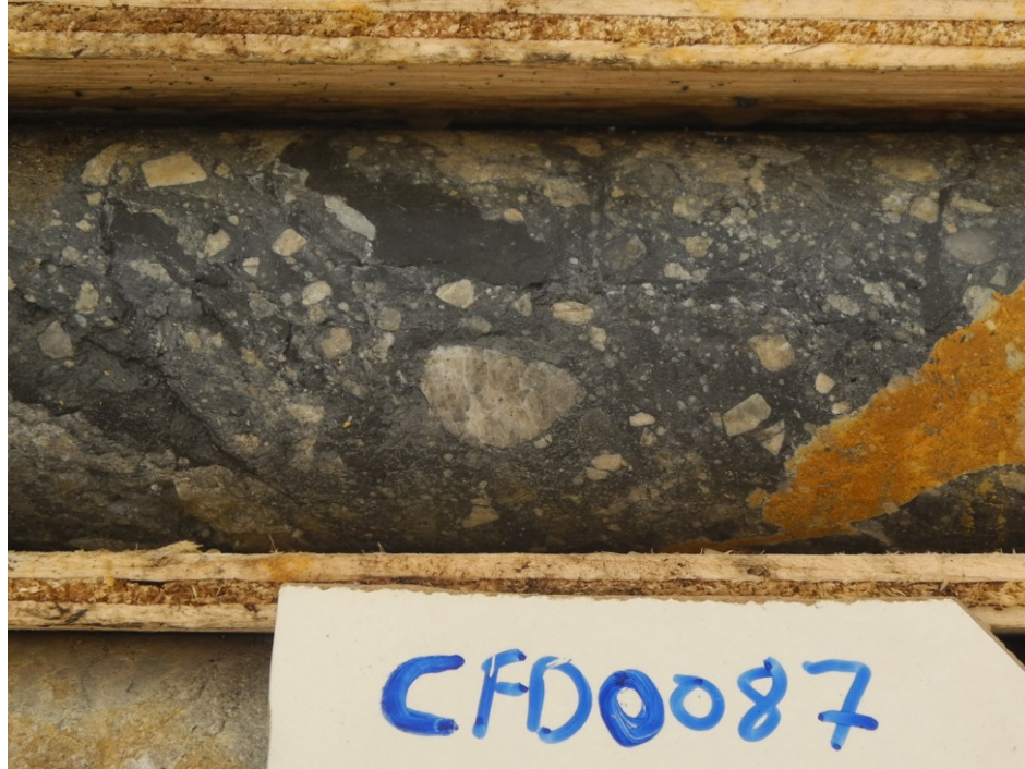
Figure 5.16: Core photograph of a sulphide-matrix breccia in drill hole CFD0087 at 130.40m down hole. Approximately 20% of the breccia matrix is composed of fine, “sooty” arsenian pyrite hosting Au.
