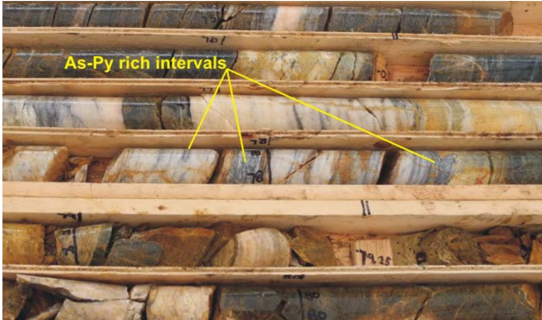
Figure 5.23: Sulphide-facies mineralization hosted within strong marble banding in CFD0079 at 78m down hole.
