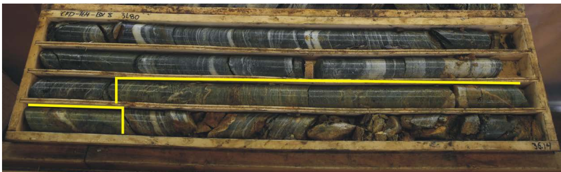
Figure 3.12: Core box photo of CFD0164 from 31.8-36.14m. The yellow marked ~1m interval is a thin and heavily altered, folded, and sheared ultramafic sliver.
