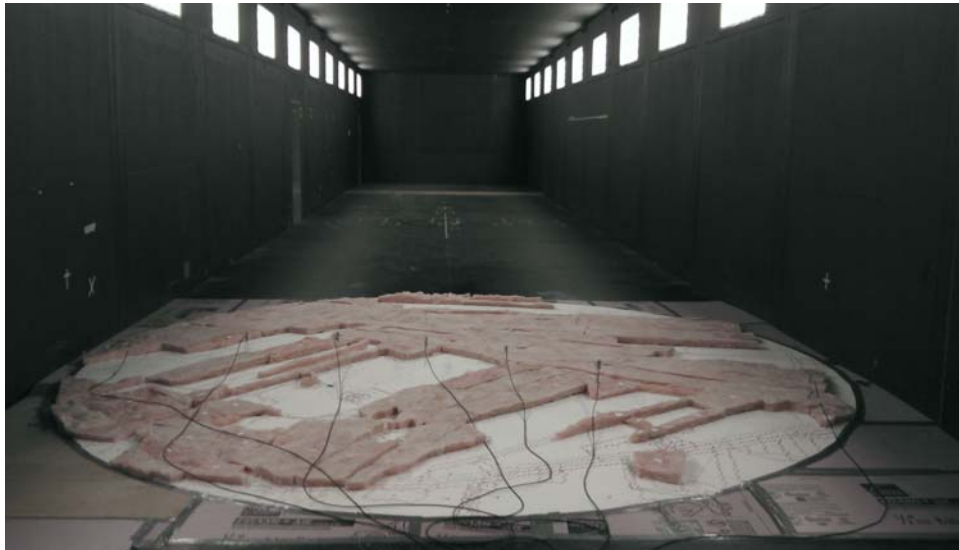
Figure 5.4: Completed wind tunnel experimental model, with attached 48% porosity forest canopy model and its placement in the wind tunnel.
