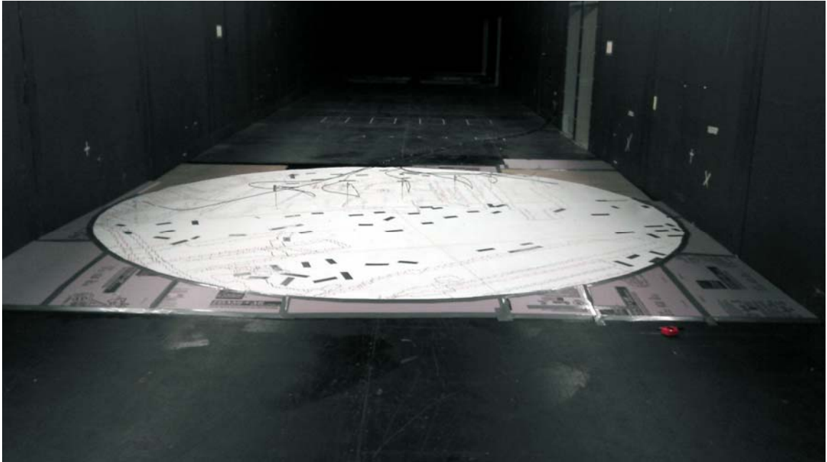
Figure D.1: Topographic model placement in the wind tunnel showing installed ramps and Cobra probes.
