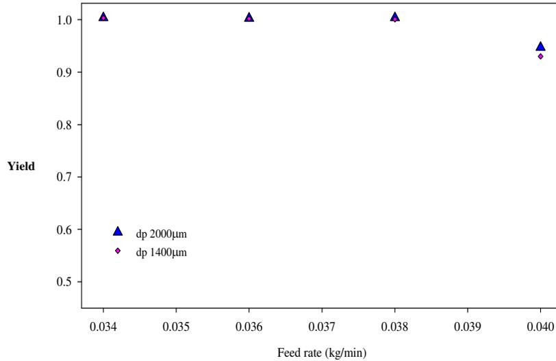
Figure 27. Effect of Particle Size on yield:  $U_{\text{seg}}=0.0963$  m/s,  $U_{\text{wm}}=0.20$  m/s,  $P_{\text{h}}=0.18$  m
