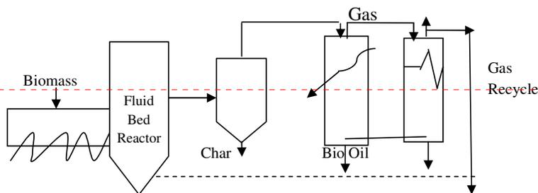
Figure 1.5. Schematic Bubbling Fluid Bed
