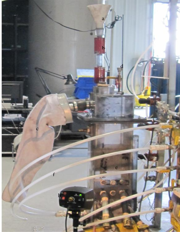
**Figure 3 Set up view of the Modified Lab scale BFB** (a-Biochar feeding inlet b-Pulsating pinch valve c-Filter bag d-Sand Inlet e-Vertical plate f-Gas sparger g-Axial Discharge Port h-light camera).
