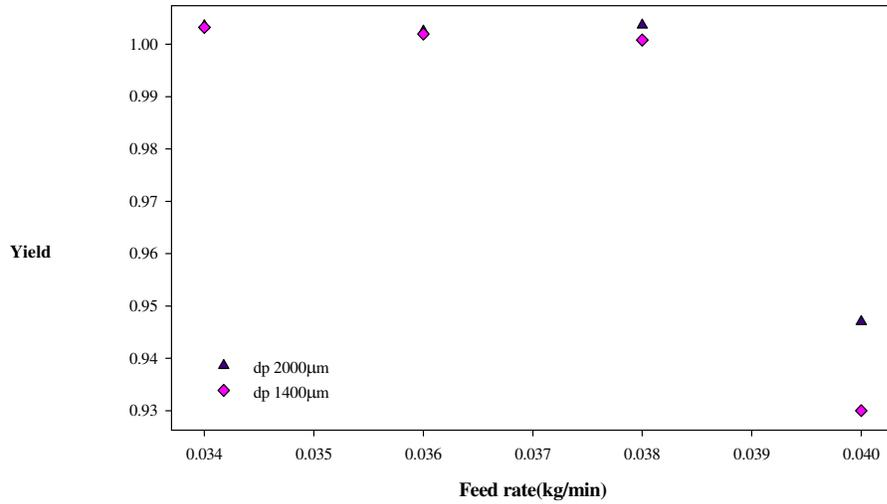
**Figure 14.** Effect of axial removal ports on yield  $U_{seg}=0.0963$  m/s,  $U_{wm}=0.20$  m/s,  $z=0.16$  m
