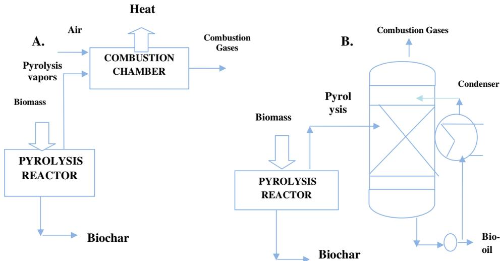
Figure 1.2. Pyrolysis Reactor for A) Biochar and Heat. B). Biochar, Bio-oil and Gases<sup>3</sup>
