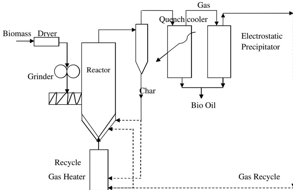
**Figure 1.3. Conceptual Representation of a Fast Pyrolysis Process**
