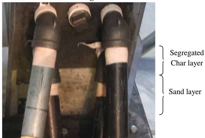
**Figure 5. Visual observation of the segregated biochar layer at steady state ( $P_h = 18$  cm,  $t = 75$  min)**
