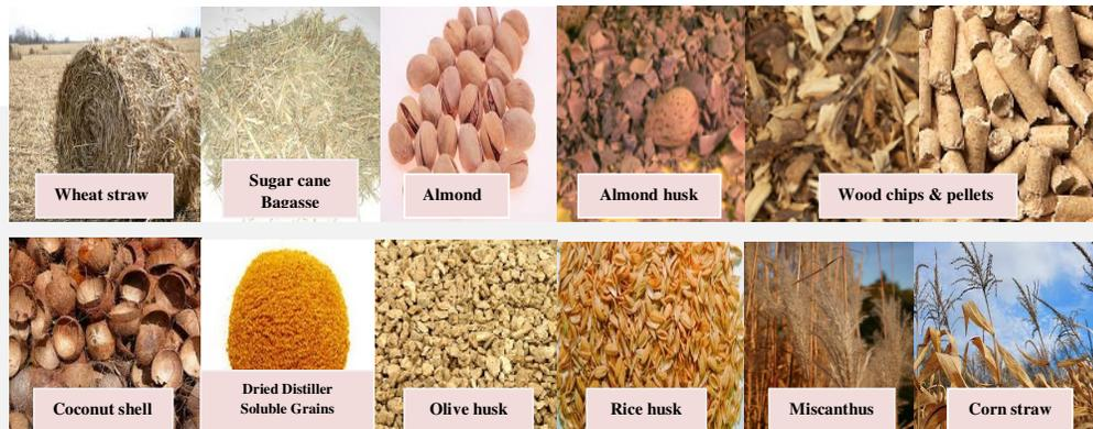
**Figure 1.1: Typical biomass of agricultural residues, forestry or woody origin used for pyrolysis**
