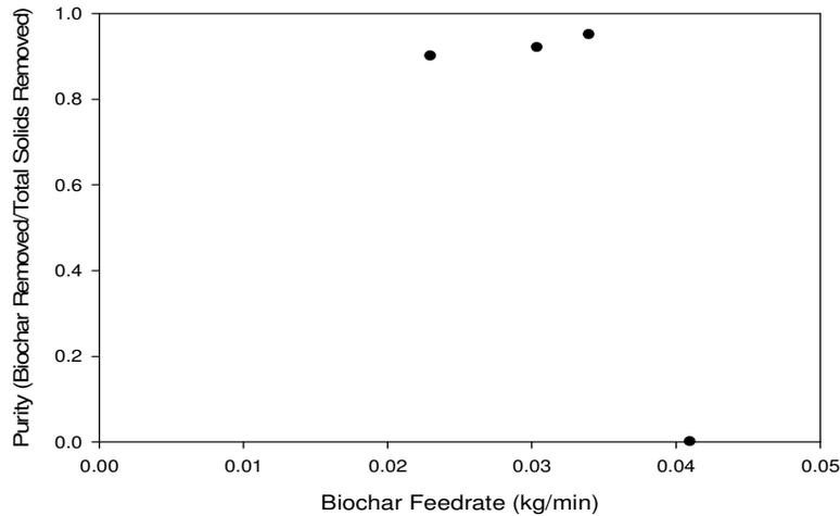
**Figure 31. Effect of biochar feedrate on purity of removal ( Mara et al, 2010)**
