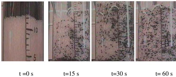
**Figure 4. Mixing profiles of biochar particles in the cold simulator Bubbling Fluidized Bed**
