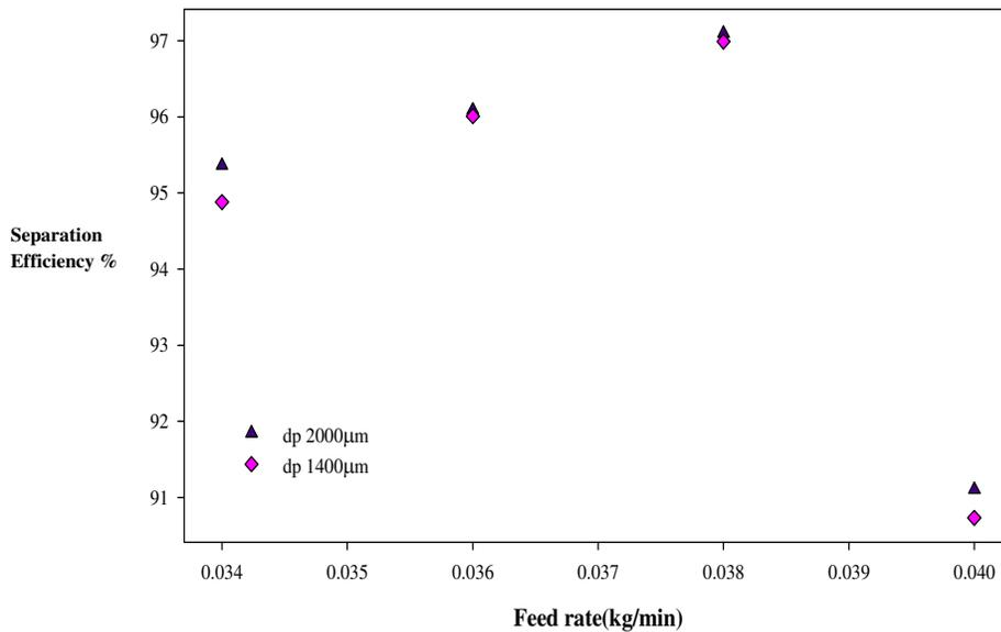
**Figure 28. Effect of Particle size on removed biochar:  $U_{seg}=0.0963$  m/s,  $U_{wm}=0.20$  m/s,  $P_h = 0.18$ m**
