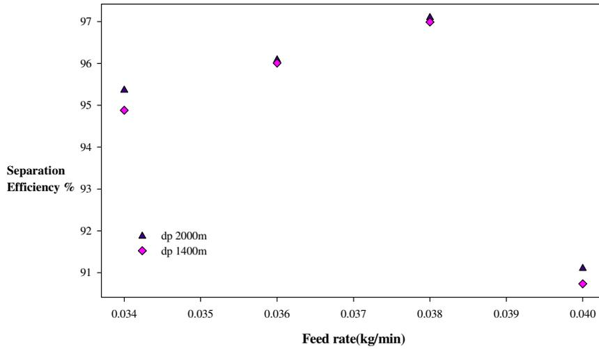
Figure 16. Effect of axial removal ports on yield  $U_{seg}=0.0963$  m/s,  $U_{wm}=0.20$  m/s,  $z=0.23$  m,  $P_h=0.18$  m
