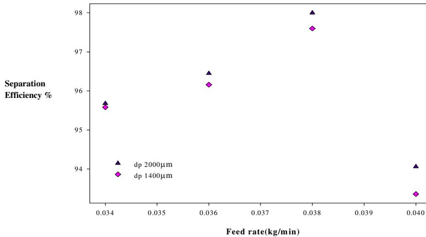
Figure 17. Comparing the effects of axial ports yield:  $U_{seg}=0.0963$  m/s,  $U_{wm}=0.20$  m/s,  $P_h=0.18$  m,  $z=0.16$  m
