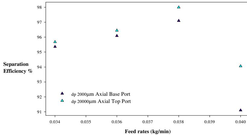
**Figure 23. Effects of axial lower port ( $z = 0.16$  m) and axial upper port ( $z = 0.23$  m) on separation efficiency**
