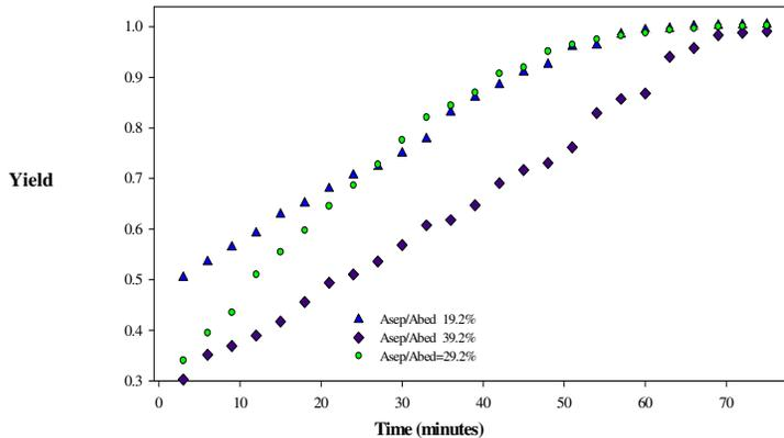
**Figure 8a. Comparing separation zones effects on efficiency  $U_{\text{seg}}=0.0963 \text{ m/s}$ ,  $U_{\text{wm}}=0.20 \text{ m/s}$**
