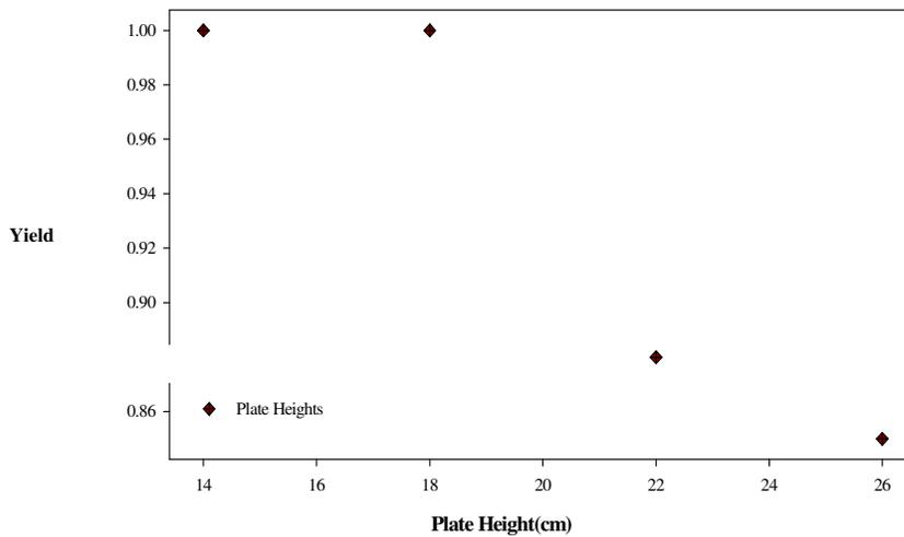
Figure 11. Biochar removal at varying plate heights at steady state,  $U_{seg}=0.09$  m/s,  $U_{wm}=0.16$  m/s
