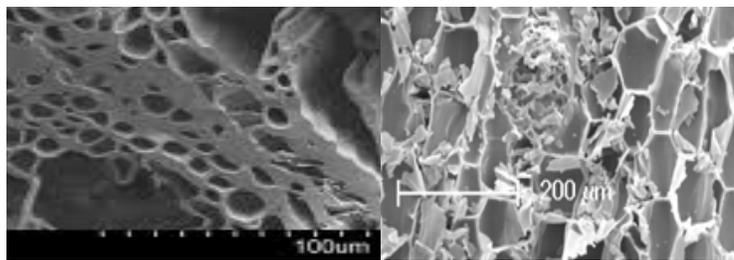
Figure 2.3. Micrograph of biochar used at 100x magnification measuring 100  $\mu\text{m}$  and 200  $\mu\text{m}$ .
