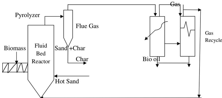
Figure 1.4. Schematic Circulating Fluidized Bed.
