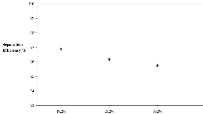
**Figure 25. Effects separation zones on biochar removed**  $U_{\text{seg}}=0.0963\ \text{m/s}$ ,  $U_{\text{wm}}=0.20\ \text{m/s}$
