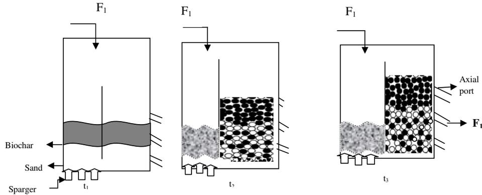
**Figure 7. Visual observation of segregated biochar layer formed with decreasing biochar in the well mixed zone and increasing biochar in the separation zone  $U_{\text{seg}}=0.0963 \text{ m/s}$ ,  $U_{\text{wm}}=0.20 \text{ m/s}$ ,  $P_h=0.18 \text{ m}$**
