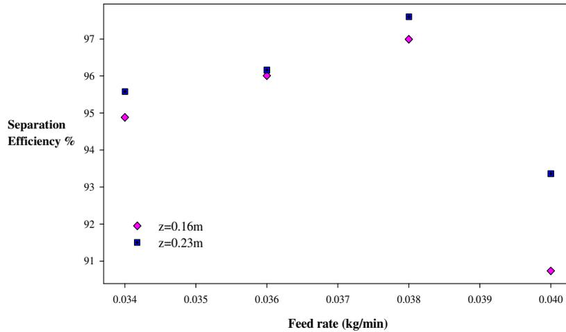
**Figure 18 Comparing effects of axial lower port ( $z = 0.16\ \text{m}$ ) and axial upper axial ( $z = 0.23\ \text{m}$ ) port on separation efficiency  $U_{\text{seg}}=0.0963\ \text{m/s}$ ,  $U_{\text{wm}}=0.20\ \text{m/s}$ ,  $P_h=0.18\ \text{m}$ ,  $d_p\ 1400\ \mu\text{m}$**
