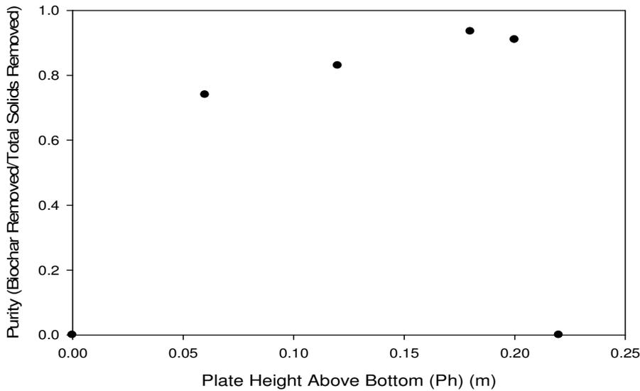
**Figure 13. Plate height effects on separation efficiency of biochar removed, Mara et.al 2010**
