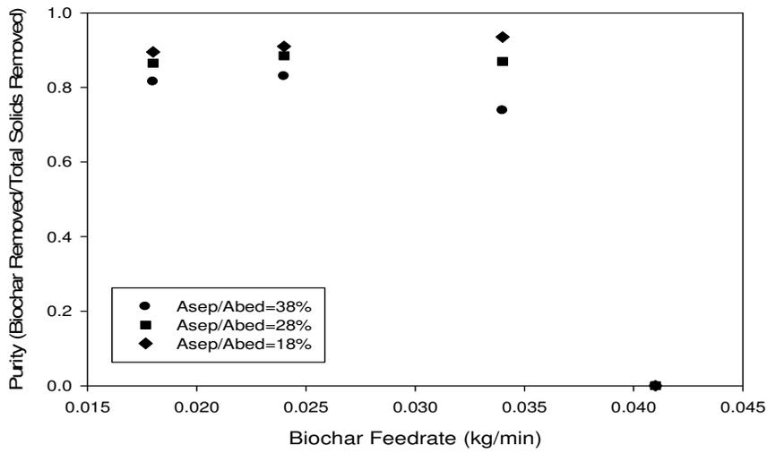
**Figure 19 Effect of separation zone on biochar separation efficiency (%), Mara 2010**
