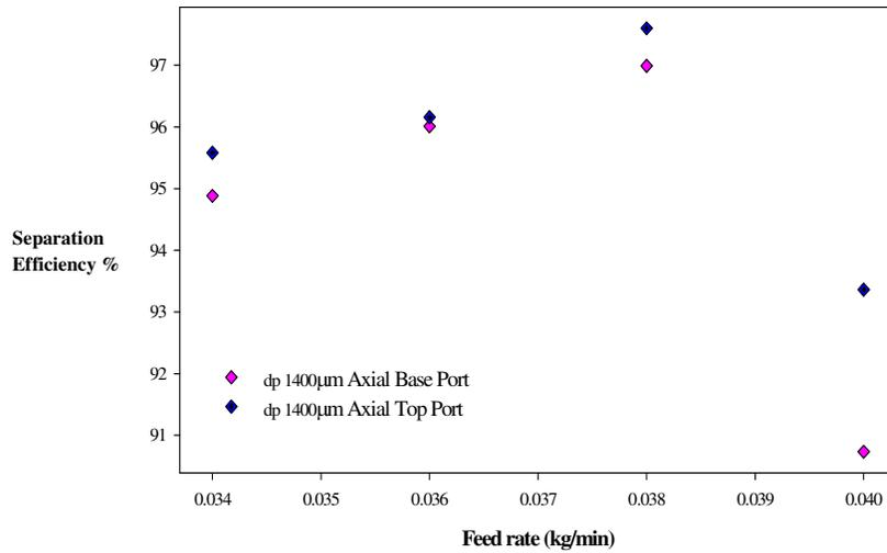
Figure 21. Axial ports effects on separation efficiency of biochar  $U_{seg}=0.0963$  m/s,  $U_{wm}=0.20$ m/s,  $P_h=0.18$ m
