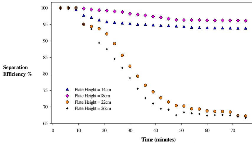
**Figure 12.** Plate heights effects on separation efficiency  $U_{seg}=0.0963$  m/s,  $U_{wm}=0.20$  m/s,  $F_{biochar}=0.036$  kg/s
