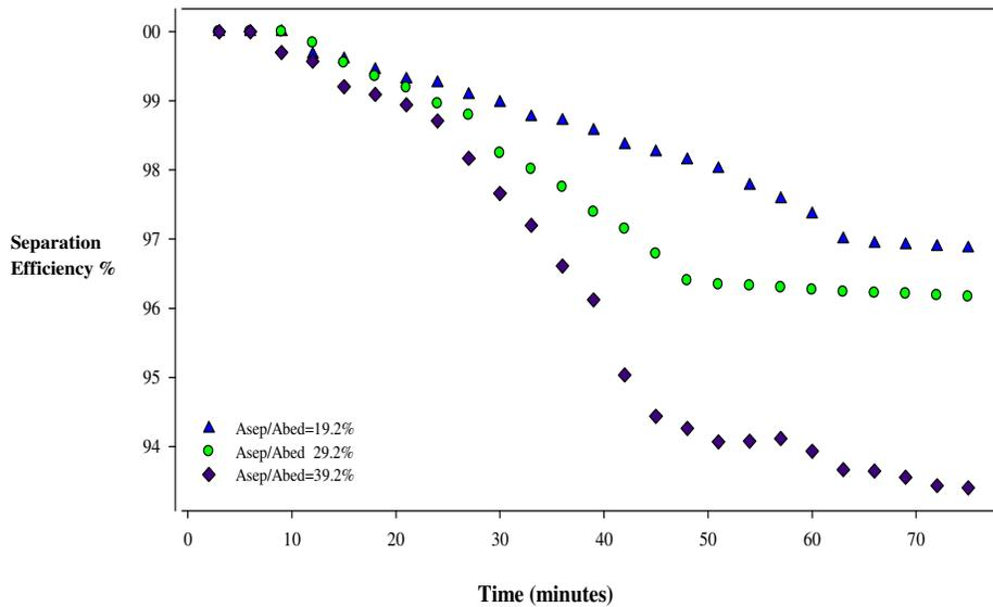
Figure 26. Comparing separation zones effects on efficiency  $U_{seg}=0.0963$  m/s,  $U_{wm}=0.20$  m/s  $P_h$  0.18m
