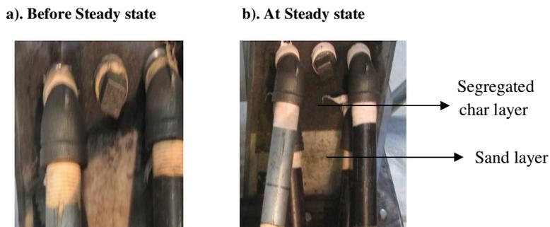
**Figure 6: Biochar Segregation before, and at steady state in a Bubbling Fluidized Bed.**
