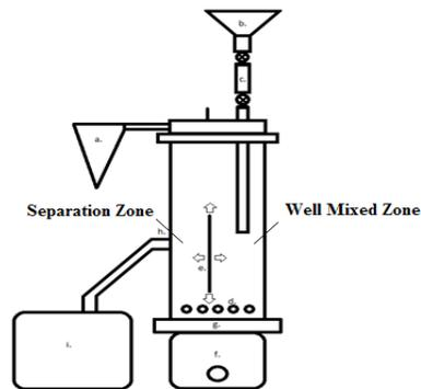
**Figure 1. Novel fluidized bed set up used for continuous biochar separation.** A) filter bag, b) solids hopper, c) biochar feed system, d) sparger distributor e) movable vertical plate f) wind box g) porous plate distributor h) removal ports. i) solids
