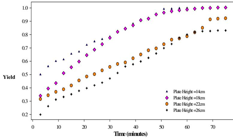
Figure 10. Biochar removal at varying plate heights (transient to steady state),  $U_{seg}=0.09$  m/s,  $U_{wm}=0.16$  m/s
