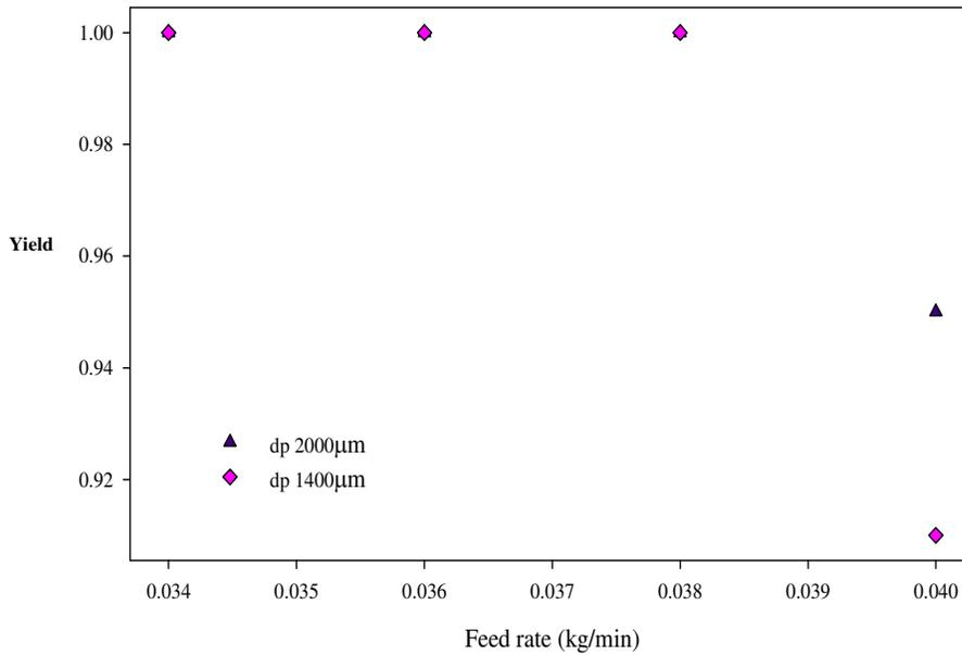
**Figure 29. Effect of Particle Size 1400 μm, 2000 μm,  $U_{seg} = 0.0963$  m/s,  $U_{wm} = 0.20$  m/s,  $z = 0.23$  m**
