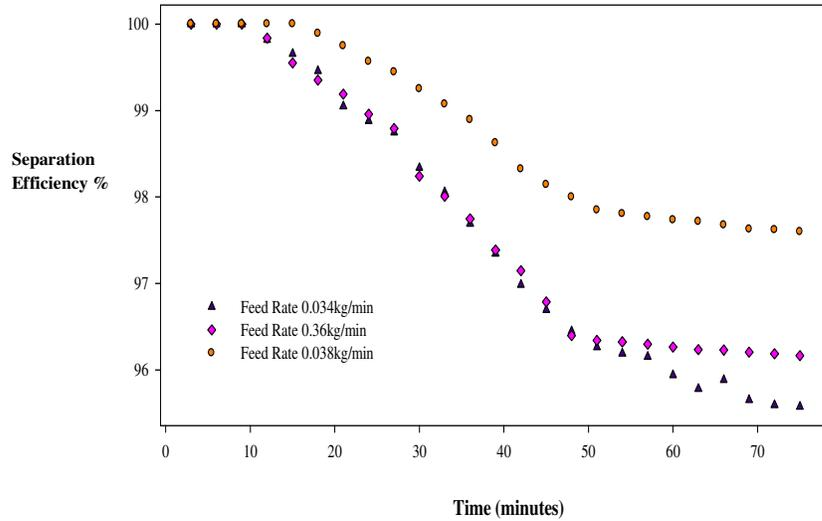
**Figure 32. Effect of biochar feed rate on separation efficiency:  $U_{seg}=0.0963$  m/s,  $U_{wm}=0.20$  m/s,  $d_p$  1400  $\mu$ m**
