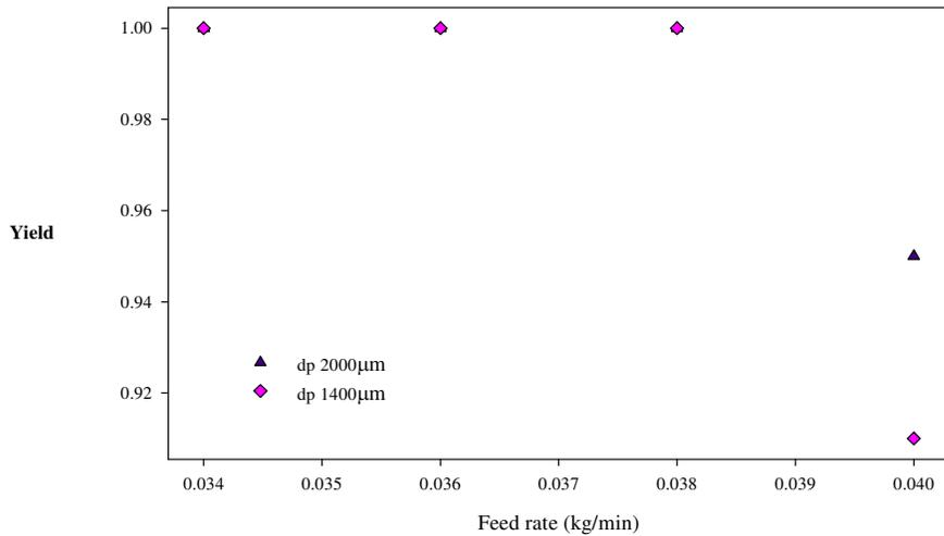
**Figure 15.** Effect of axial removal ports on yield  $U_{seg}=0.0963$  m/s,  $U_{wm}=0.20$  m/s,  $z=0.23$  m
