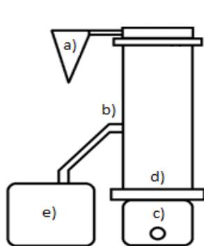
**Figure 2. Fluidized bed used for segregation and removal experiments:**
