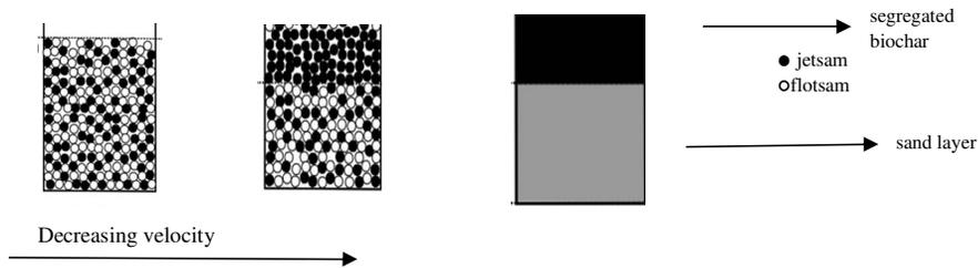
**Figure 1.6. Representation of mixing and segregation processes of dissimilar solids**
