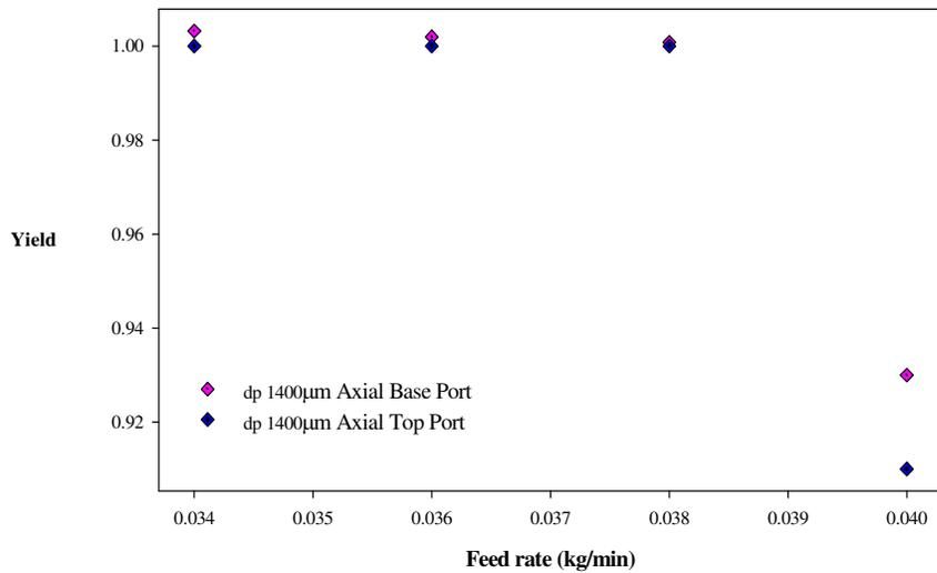
**Figure 20. Comparing effects of axial ports)  $U_{seg} = 0.0963$  m/s,  $U_{wm} = 0.20$  m/s,  $P_h = 0.18$  m,  $d_p = 1400$  µm**
