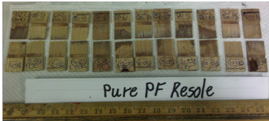
Figure 5- 7: Test specimens after failure for pure PF resole synthesized with F/P of 2.1 (wood failure)
