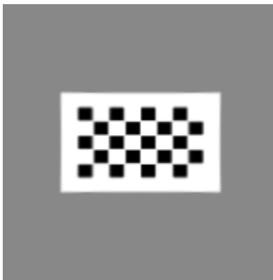
Figure 1-5: The distorted image corrected with coefficients (-10, -100, -1000) for the radial distortion correction equation applied.
