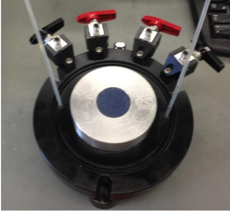
1) – Enlarged platen over the pedestal
