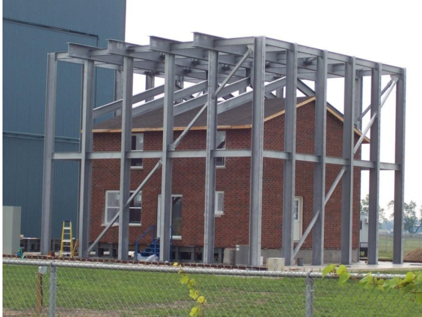
Figure 2.1: Full-scale experimental set-up with steel reaction frame (source: http://www.eng.uwo.ca/irlbh/ )
