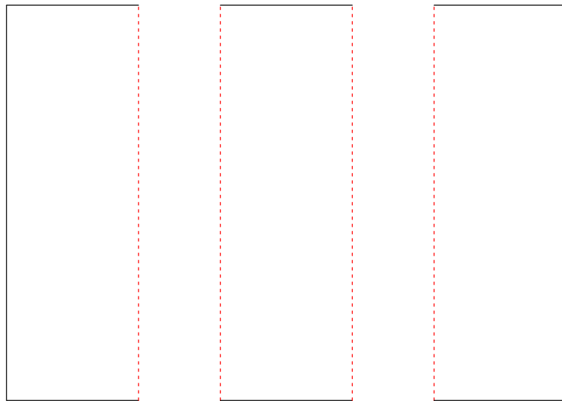
Figure 3.8: When applying edge correction in parallel computation of spatial statistics, each processor is aware of only the extent of its own sub-window, yet needs to be aware of whether a boundary is a global boundary (black) and requires edge correction, or an interior boundary (red) that requires no edge correction.
