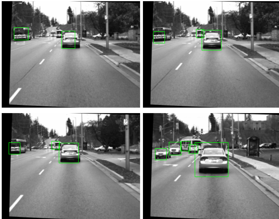
Figure 2.10: Real-time vehicle tracking experiment using the RoadLAB instrumented vehicle in i-ADAS mode
