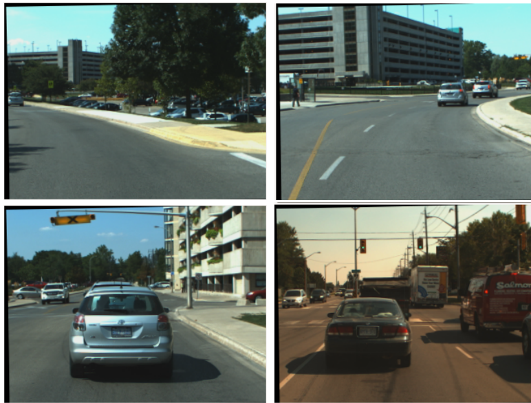
Figure 3.1: Challenges of lane detection: a) (top-left): different curvature and shapes b) (bottom-left): vanished lane markers c) (top-right): splitting and merging lanes d) (bottom-right): occlusion and clutters
