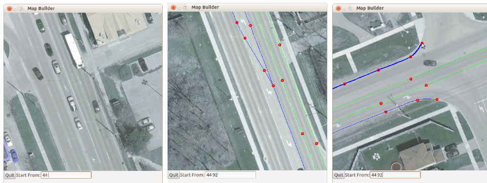
Figure 3.3: Images from the map building application a) (left): visible lanes in presence of traffic b) (center): Splitting lane sample c) (right): Several neighboring lanes
