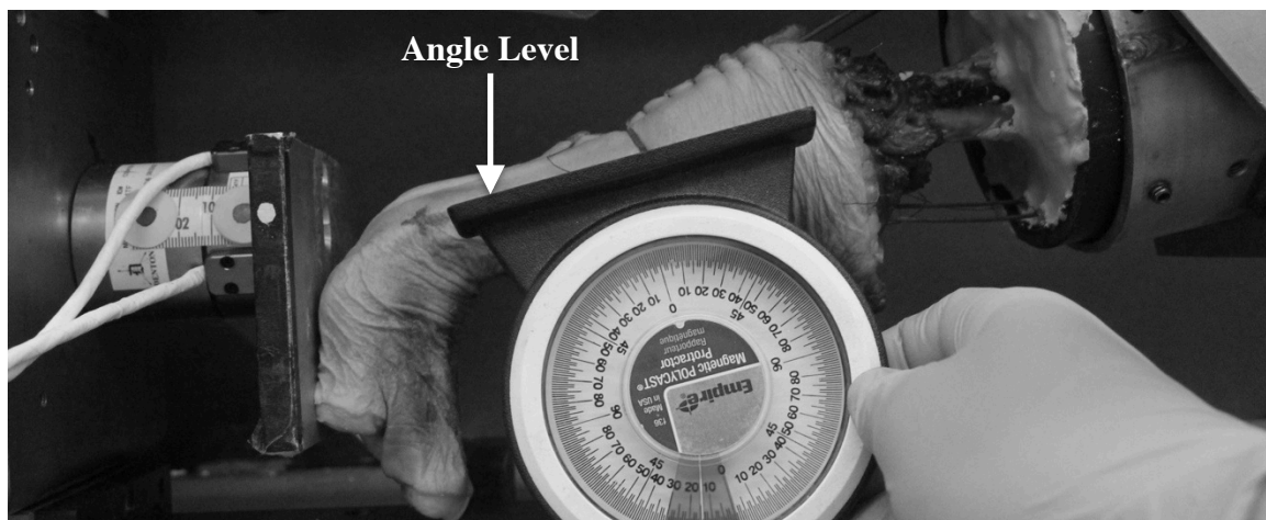
Figure J.14: Specimen orientation prior to impact
