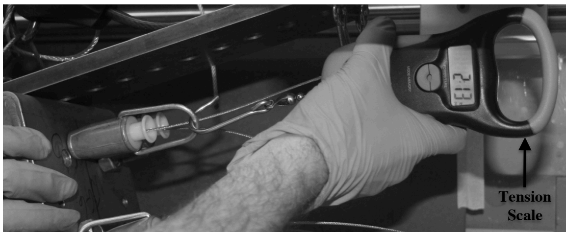
Figure J.16: Tendon load measurement
