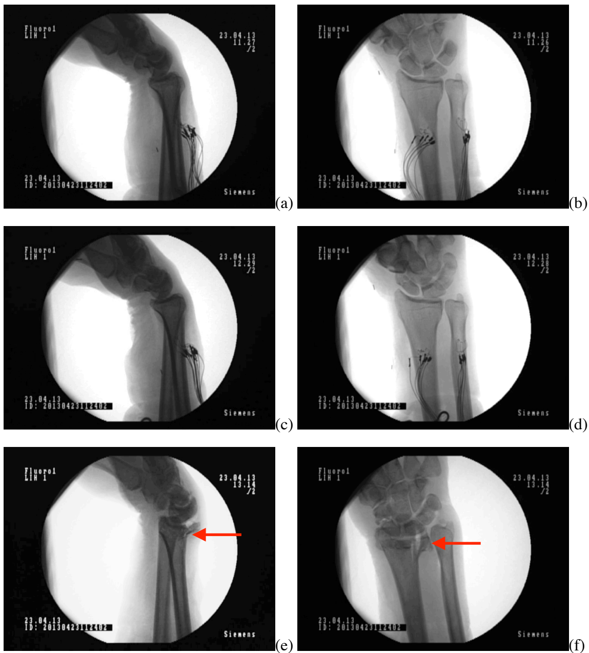
Figure K.5: Pre-fracture lateral (a) and anterior-posterior (b) digital radiographs, Intermediate lateral (c) and anterior-posterior (d) digital radiographs, and fracture lateral (e) and anterior-posterior (f) digital radiographs for specimen 12-07016L
