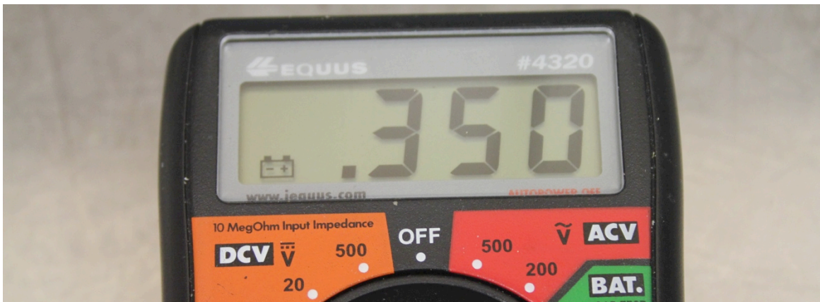
Figure J.23: The multi-meter resistance should match the number on the gauge packaging. A higher number implies that there is not a good connection, while a lower number implies that the gauge is shorting out
